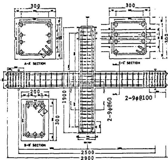
Fig.6 Specimens Tested by Kamimura et al. [31]
