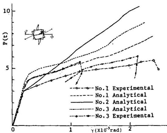
Fig.14 Load-Joint Distortion Relationships
