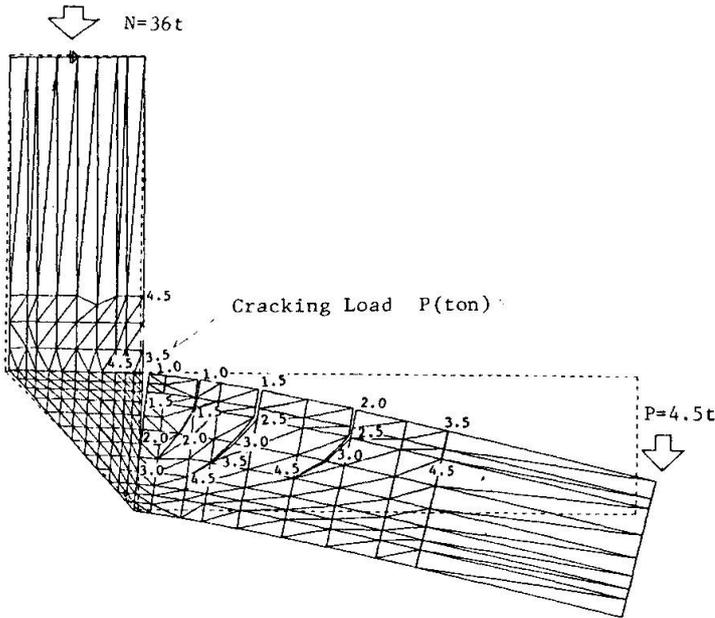
Fig.9 Crack Propagation for No.1(P=4.5t)
