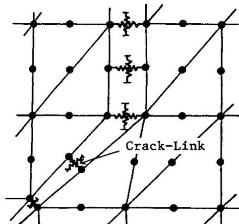
Fig.5 Crack-Link Elements
