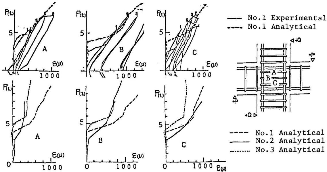
Fig.19 Relationships between Load and Strain of Ties
