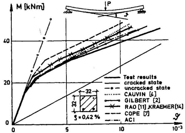
Fig.6: Rotation of support sections as a function of maximal moment for beam 1.13 of EIFLER, PLAUK [16]
