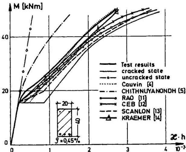
Fig.5: Moment-curvature relationship for beam 4 of CLARK, SPEIRS [1]
