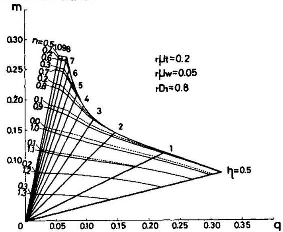
Fig.6 Nondimensional Interaction Curves between Bending and Shear
