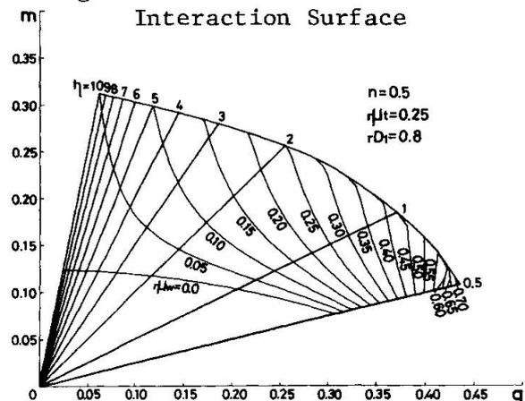
Fig.8 Nondimensional Interaction Curves between Bending and Shear
