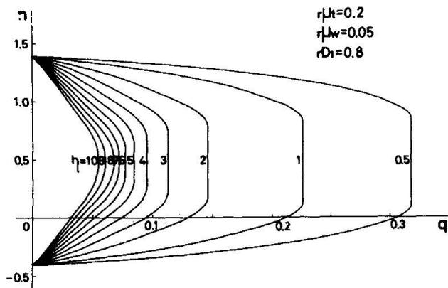
Fig.5 Nondimensional Interaction Curves between Compression and Shear
