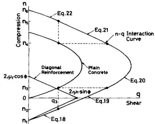
Fig.10 Method of Superposition.
