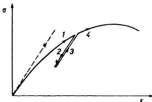
Figure 8 Loading - Unloading
