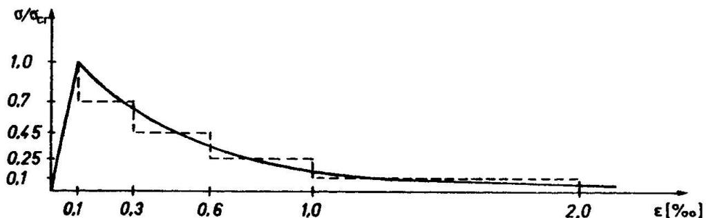
Figure 6 Stresses in the concrete after cracking
