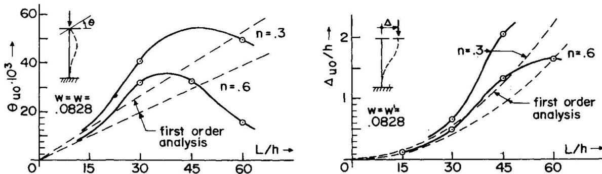
Fig. 11 Short Term Rotation and Displacement Capacities
