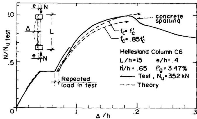
Fig. 5 Comparison with Test Data [7,8]
