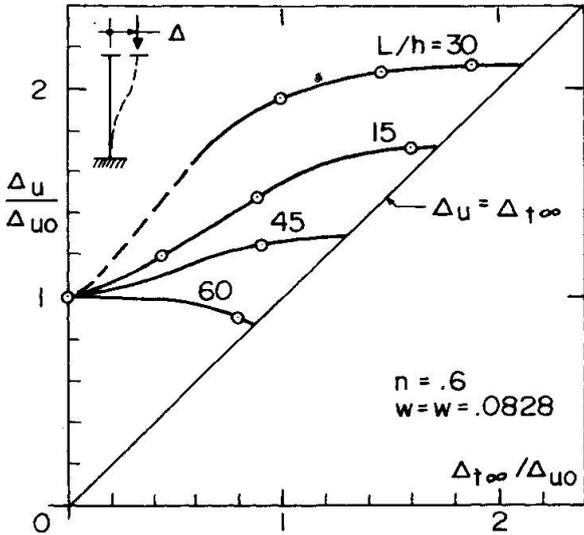
Fig. 13 Total Displacement Capacity versus Long Term Displacement
