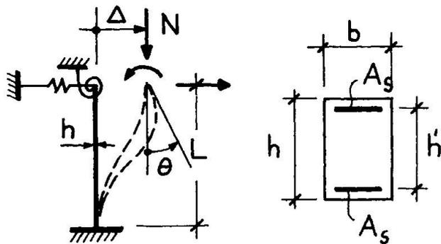
shortening due to axial loading, the columns considered are fixed at both ends. This is achieved by assigning spring constants to the spring restraints (Fig. 6) that are several order of magnitudes larger than the rotational or translational column stiffness. External forces at the column top, required to produce a specified end rotation or displacement, are therefore a function of the spring constants alone.
