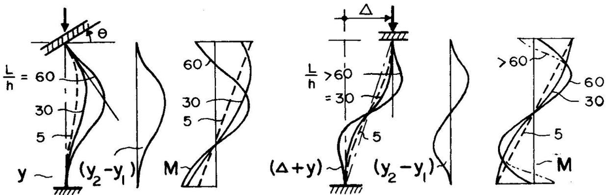
Fig. 10 Schematic Short Term Deflection and Moment Distributions at Failure ( $n \sim 0.6$ ;  $w \sim .08$ )
