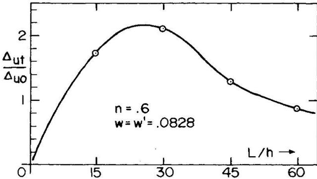
Fig. 14 Long Term Displacement Capacity versus Slenderness Ratio
