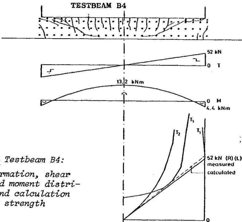
Fig. 2.5 Testbeam B4:
