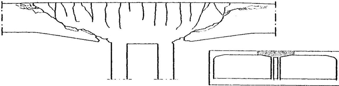
*Fig. 2.1 Part of a tunnel-section after testing*
