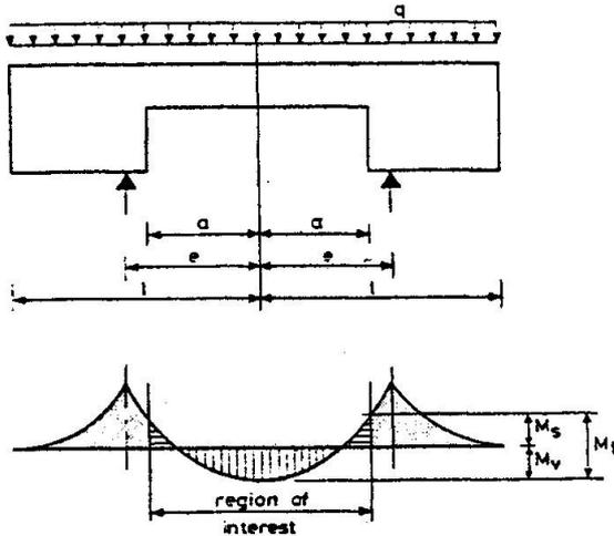
Fig. 2.2 Test-specimen
