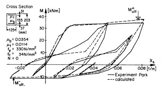
Fig. 8 Comparison III between FE-Calculation and Experiment [2]
