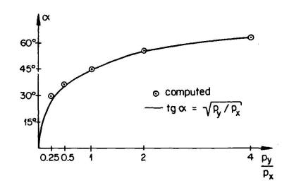
Fig. 18 Analytical and Computed Values of  $\alpha$
