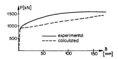
Fig. 13 HEM-160, Beam A3 [5]  $f_{y} = 360 \text{ N/mm}^{2}$  $f_{11} = 540 \text{ N/mm}^{2}$
