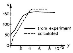
Fig. 19 Shear Force - Shear Strain
