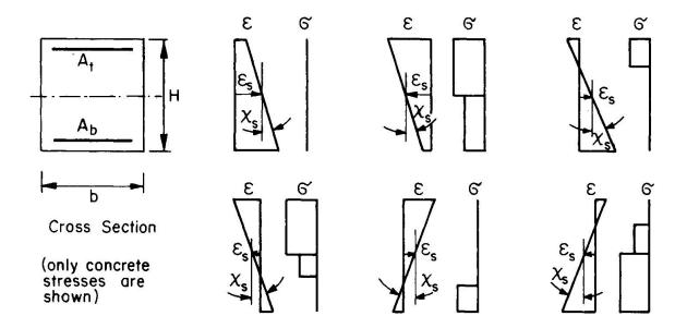
Fig. 2 Strain and Stress Distributions
