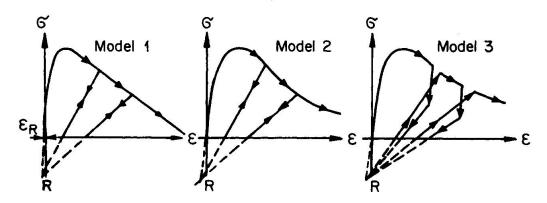
Fig. 5 Typical Stress-Strain-Relationship of Concrete Models
