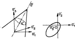
Fig. 10 Drucker-Prager (extended v. Mises) Yield Criterion
