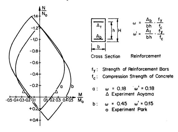
Fig. 4 Interaction Curves (rigid plastic material)
