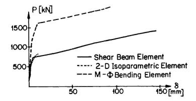
Fig. 15 Frame Displacements at Failure
