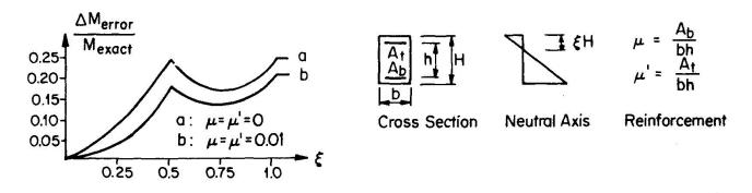
Fig. 3 Accuracy for the Stringer Model (linear elastic material)
