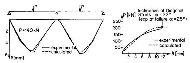
Fig. 21 Displacements of Beam HH5 [8]
