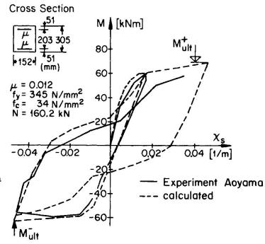
Fig. 7 Comparison II between FE-Calcultation and Experiment [2]
