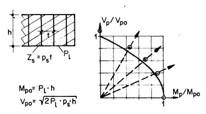
Fig. 20 Bending Moment - Shear Force Interaction Diagram
