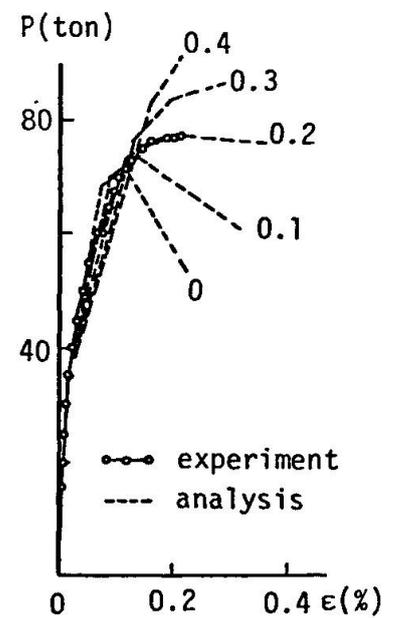
Fig. 21 Loads vs. Strain of Hoop
