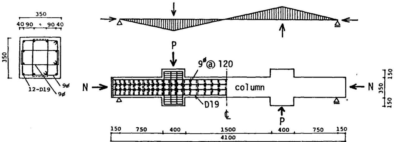
Fig. 22 Test Column (by Hisada, Ohmori and Bessho)
