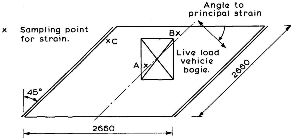
Fig. 1 Model Skew Slab
