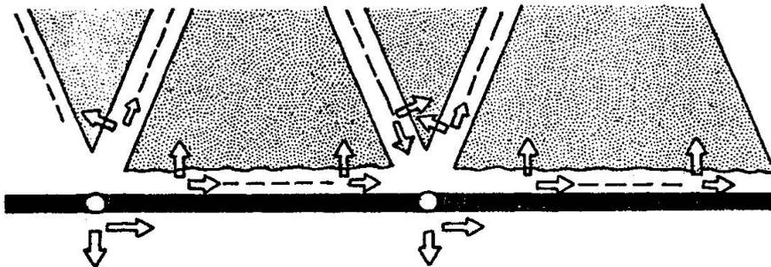
*Fig. 2 Special type of reinforcement bar element in the equilibrium model with natural boundary displacements*
