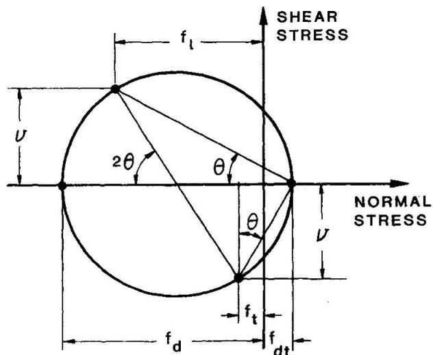
Fig. 17 Equilibrium Conditions for Average Stresses in Concrete
