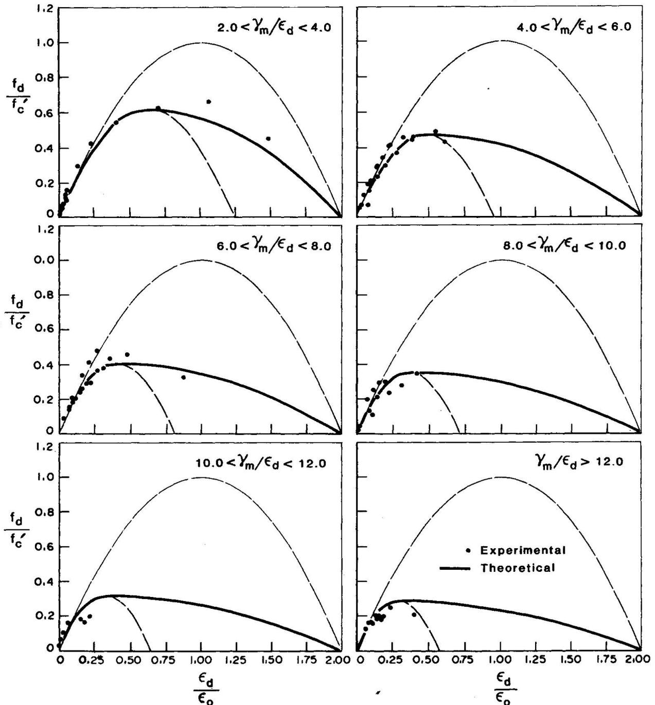
Fig. 14 Influence of Shear Strain on Principal Compressive Stress-Strain
