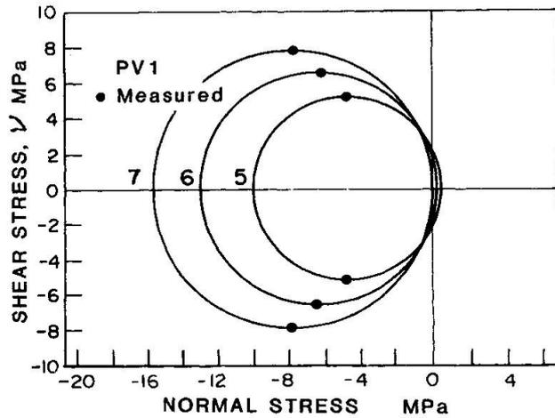
Fig. 12 Mohr's Circles of Stress for Specimen PV1
