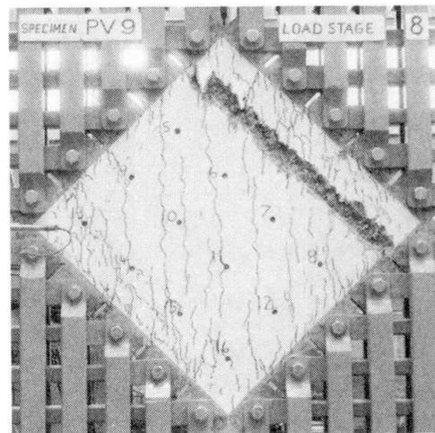
Fig. 5 Specimen PV9: Sliding Shear Failure of Concrete
