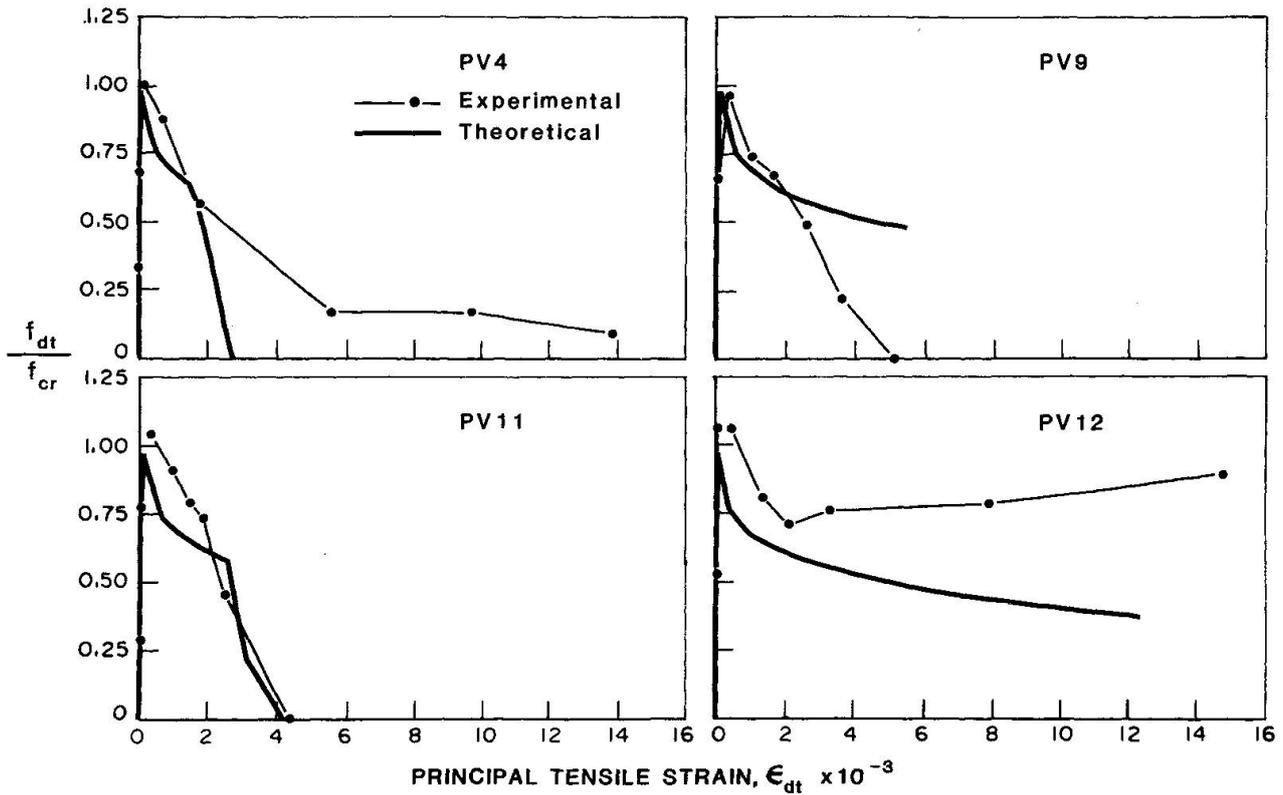
Fig. 15 Principal Tensile Stress-Strain Behaviour of Concrete
