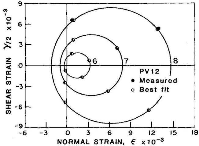
Fig. 11 Mohr's Circles of Strain for Specimen PV12
