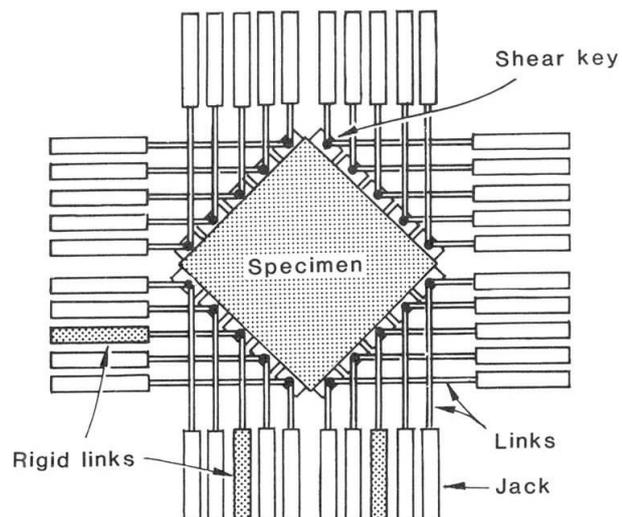
Fig. 2 Hydraulic Jack and Link Assembly
