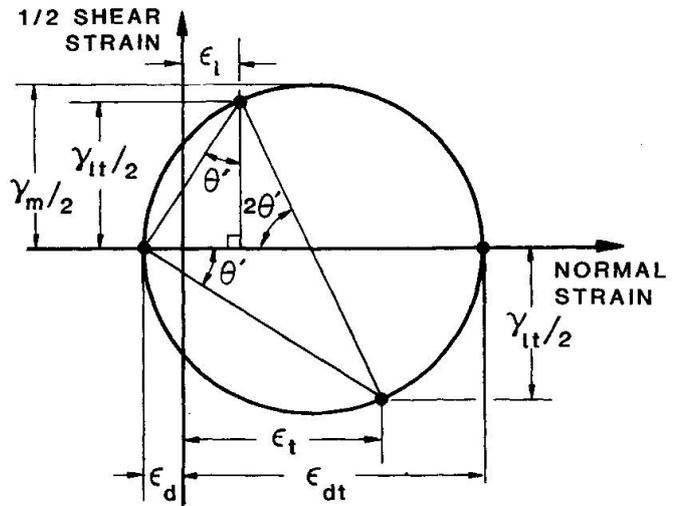
Fig. 18 Compatibility Conditions for Average Strains in Concrete
