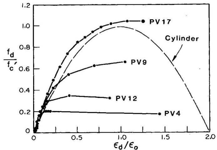
Fig. 13 Principal Compressive Stress vs. Principal Compressive Strain
