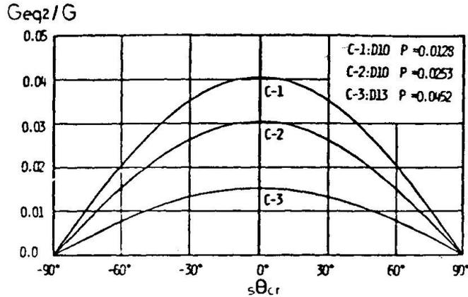
Fig.15 Equivalent Shear Stiffness due to Dowel Action
