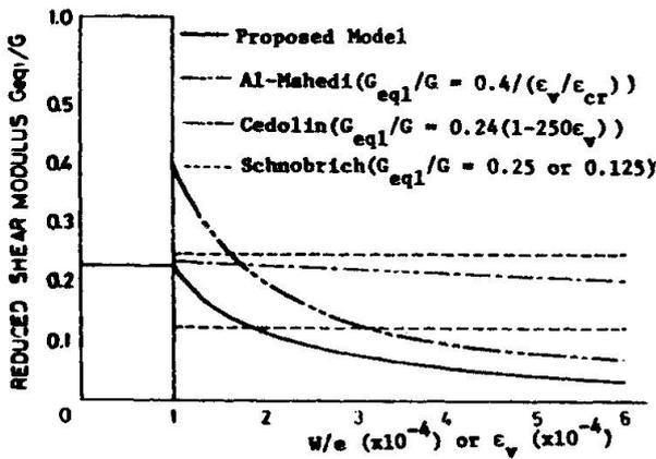
Fig. 11 Shear Stiffness Reduction in Cracked Concrete
