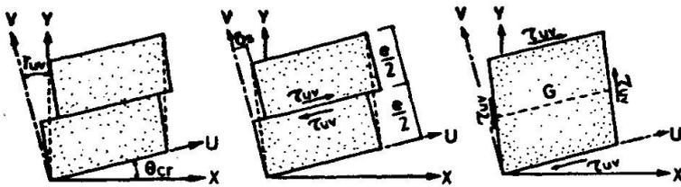
Fig. 9 Assumed Shear Strain for Cracked Concrete
