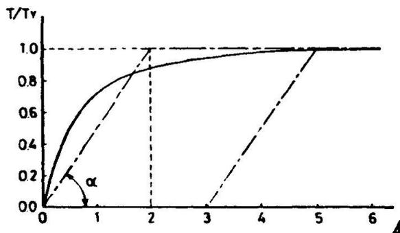
Fig.13 Non-Dimensionized Dowel Force Curve
