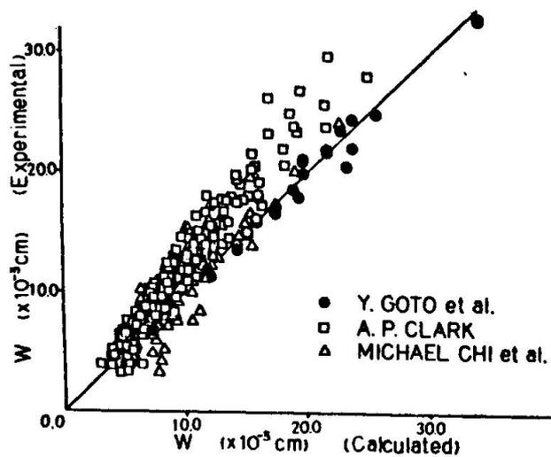
Fig.19 Comparison between Calculated and Experimental Crack Widths
