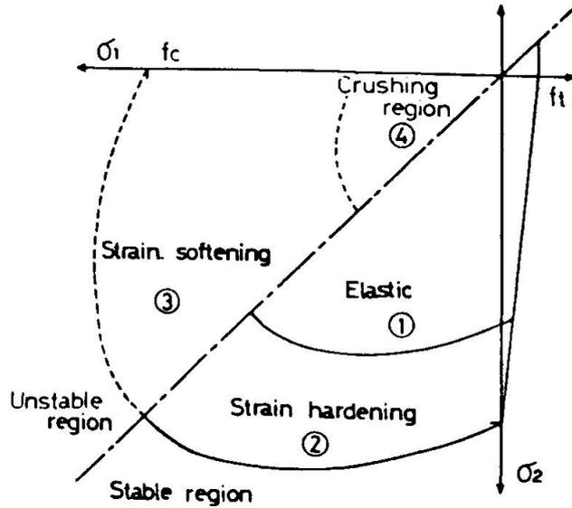
Fig.2 Assumed Fracture and Yield Surfaces of Concrete
