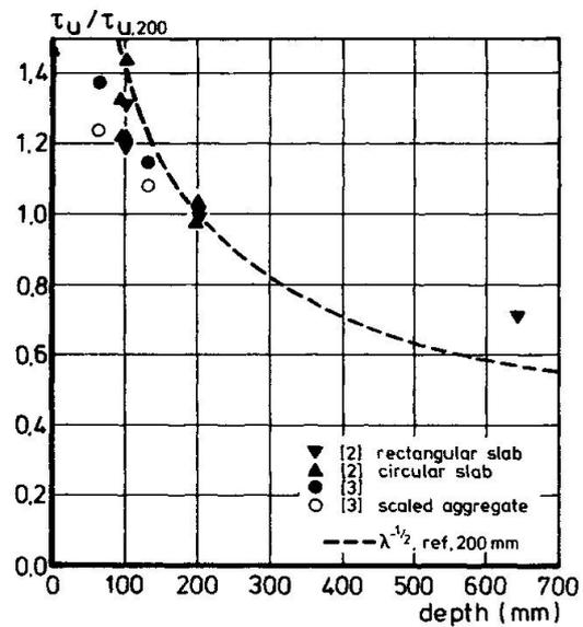
Fig. 5. Relative ultimate shear stress vs. depth of the beam
