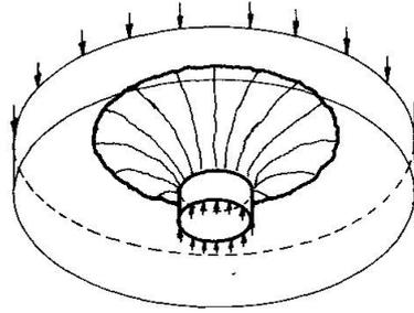
Fig. 2. Punching shear of concrete slab
