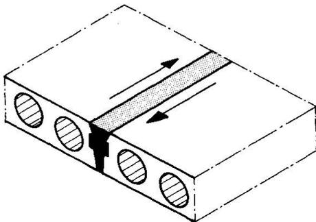
Fig. 3. Hollow core slab with mortar joint
