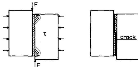
Fig. 4. Shear stresses and crack in the joint
