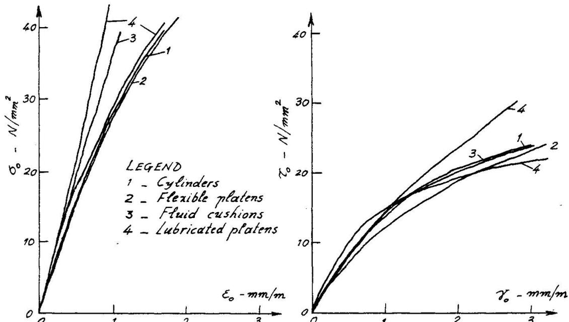
Fig. 2 Volumetric ( $\sigma_0 - \epsilon_0$ ) and deviatoric ( $\tau_0 - \gamma_0$ ) stress-strain relationships for concrete under triaxial compression obtained from tests using various friction reducing techniques
