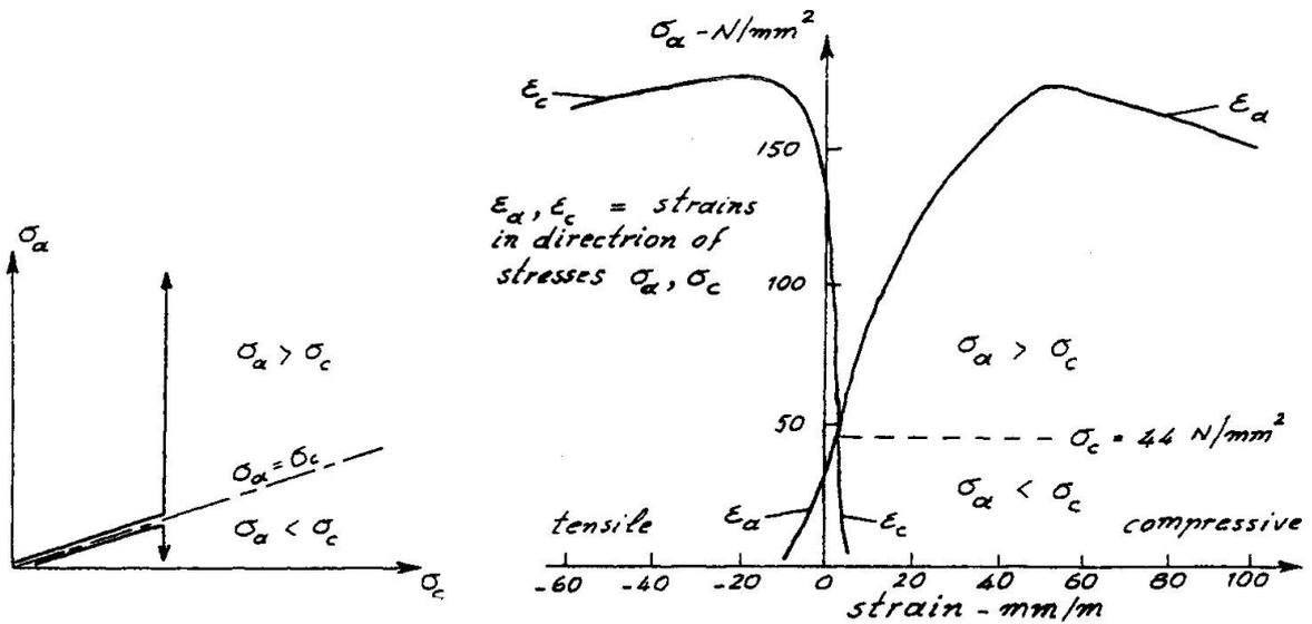
Fig. 10 Stress path used in triaxial tests
