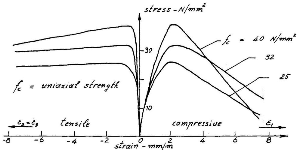
Fig. 3 Stress-strain relationships for concretes under uniaxial compression obtained from tests on cylinders
