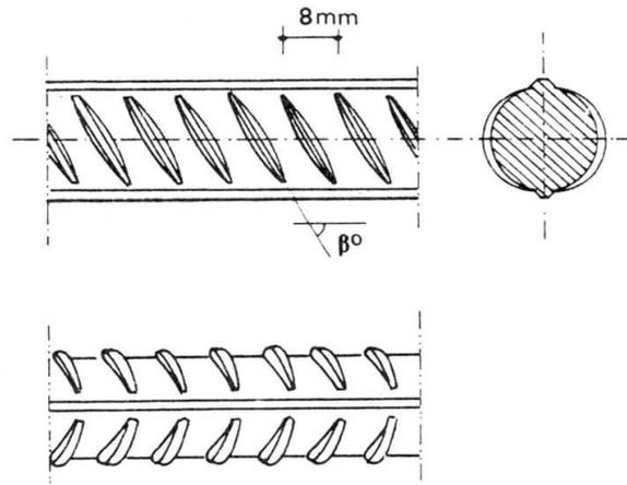
Fig. 2-a Geometrical characteristics of the deformed bar used in the tests
