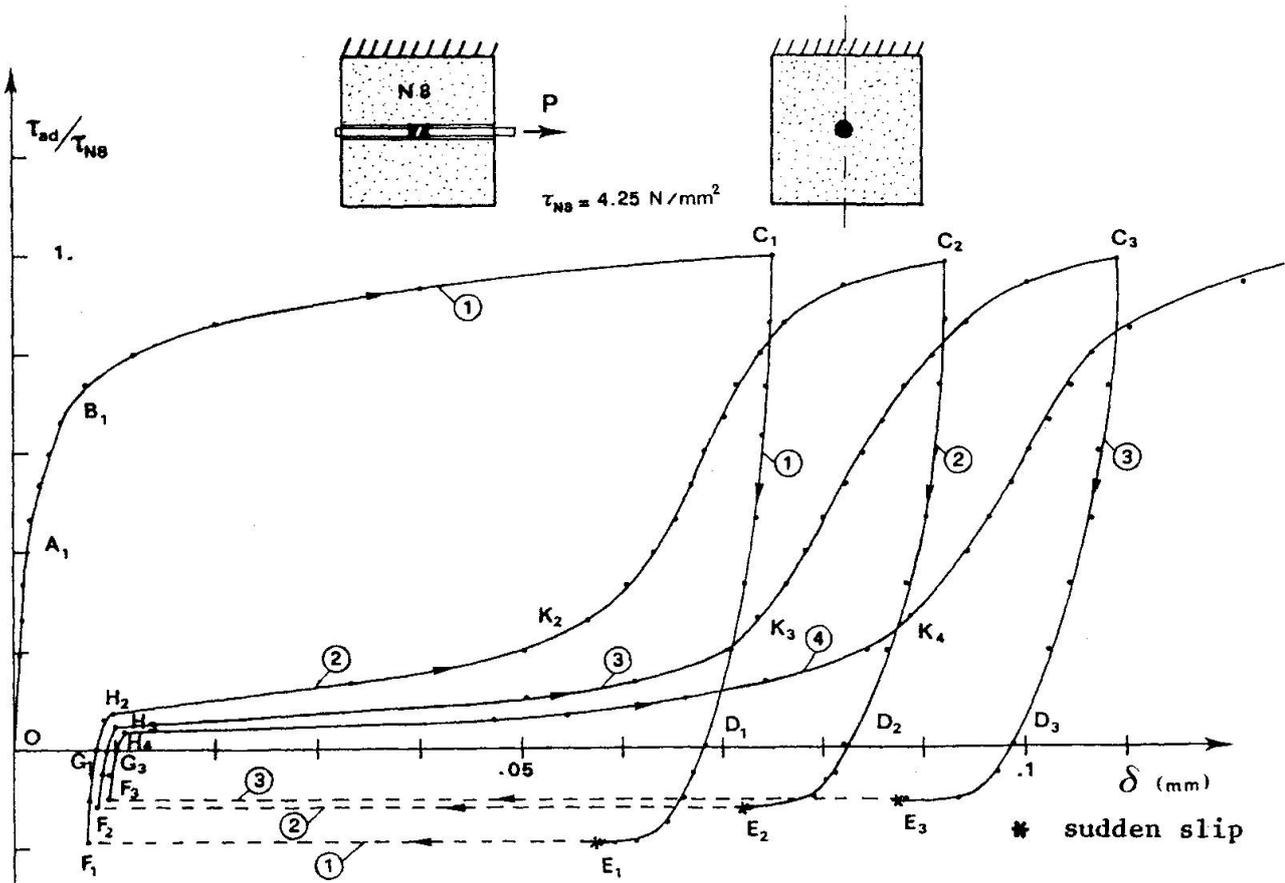
Fig. 8 - Bond-slip curves with cyclic loading (the maximum bond stress is kept constant in each cycle)
