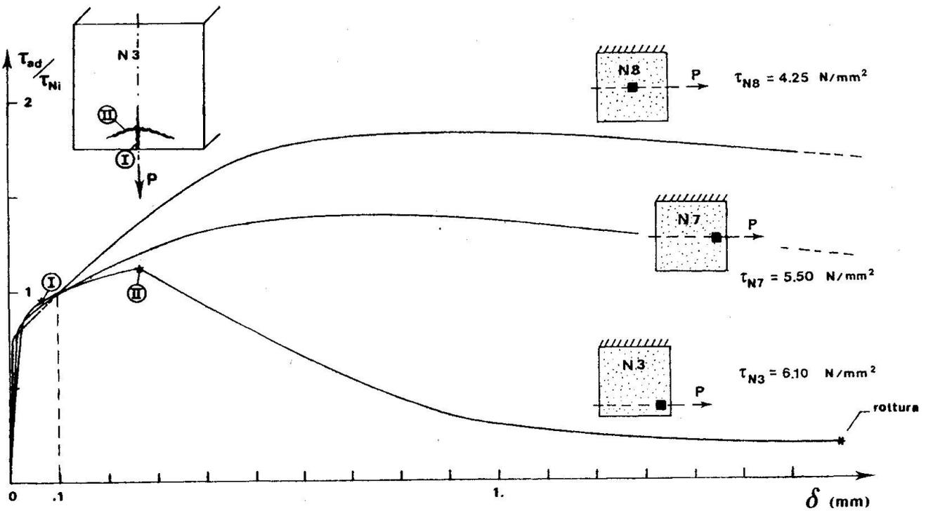
Fig. 19-a - Bond-slip curves for large displacements
