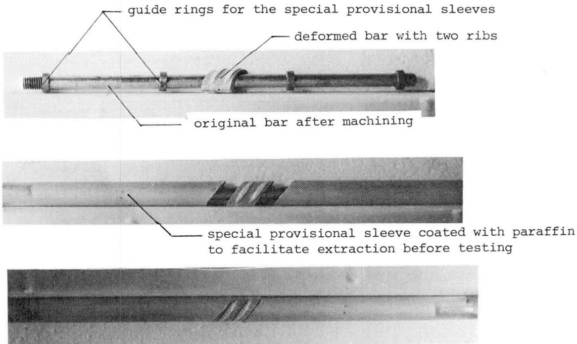
external aspect of the test bar before concrete casting, with the provisional sleeves closed up to the ribbed element
