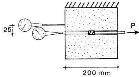
Fig. 3-d - Instruments to measure slip
