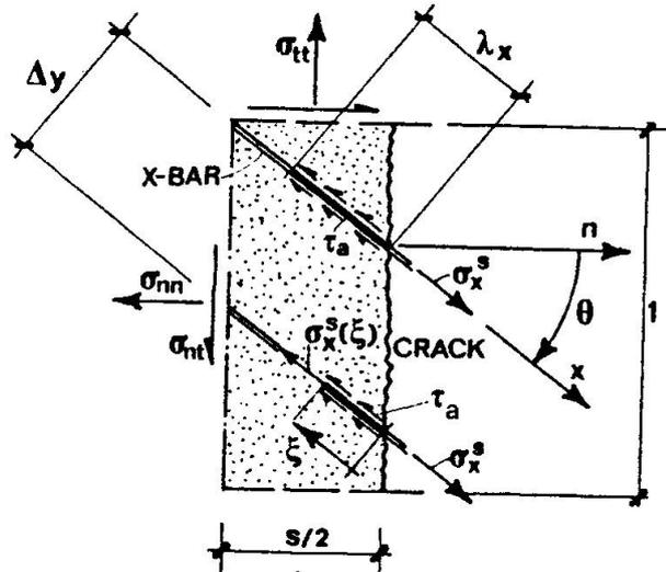
Fig.12-Concrete stresses between two contiguous cracks.
