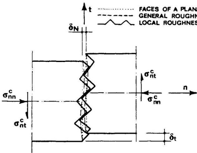
Fig.1 - Crack morphology.
