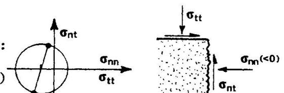
The crack slip must always have the same sign as  $\sigma_{nt}$ : otherwise, when the value of the slip goes back to zero, the internal force  $\sigma_{nn}$  ought to become positive (i.e. tensile), because in this situation ( $\delta_t = 0, \delta_n > 0$ )
