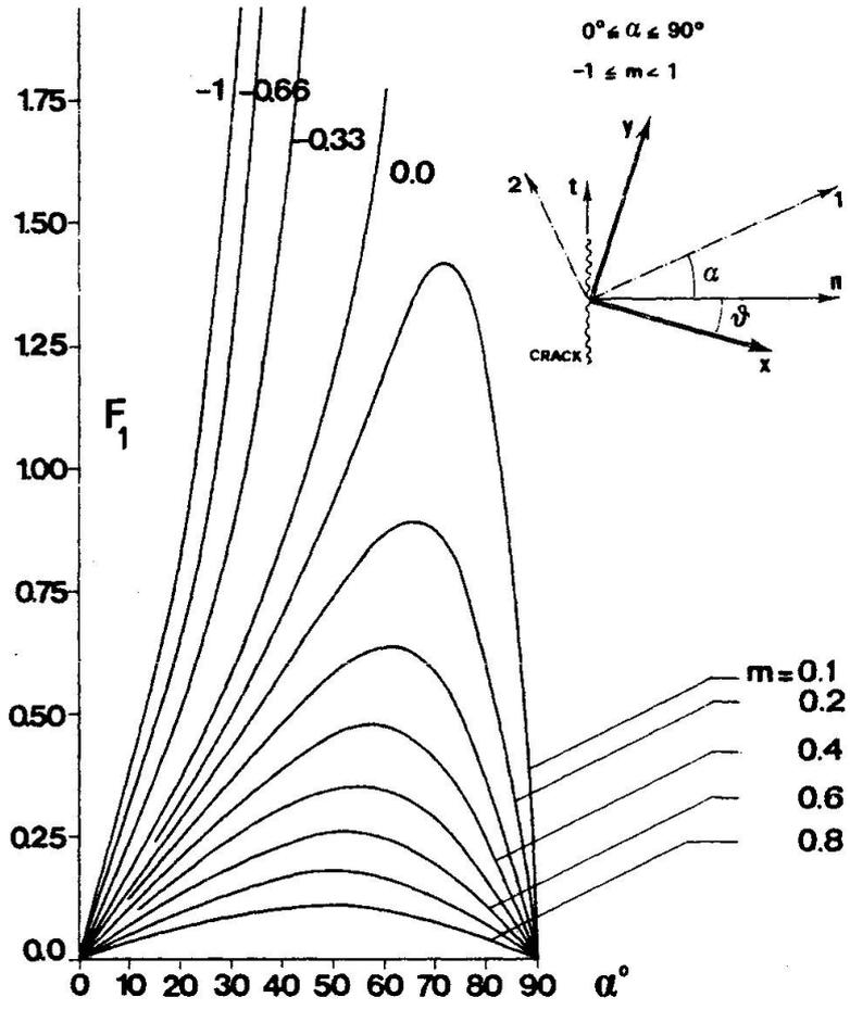
Fig. 6b - Plot of the function  $F_1$  for various values of the ratio  $m$  between the principal stresses.
