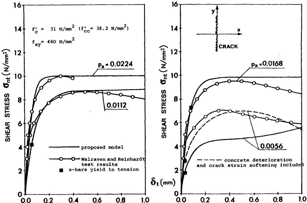
Fig.17 - Fit of Walraven and Reinhardt's results, steel tension stiffening included, for a medium strength concrete (crack spacing  $s = 50 \text{ mm}$ , bond length of the bars in the experimental tests  $L = 400 \text{ mm}$ ).
