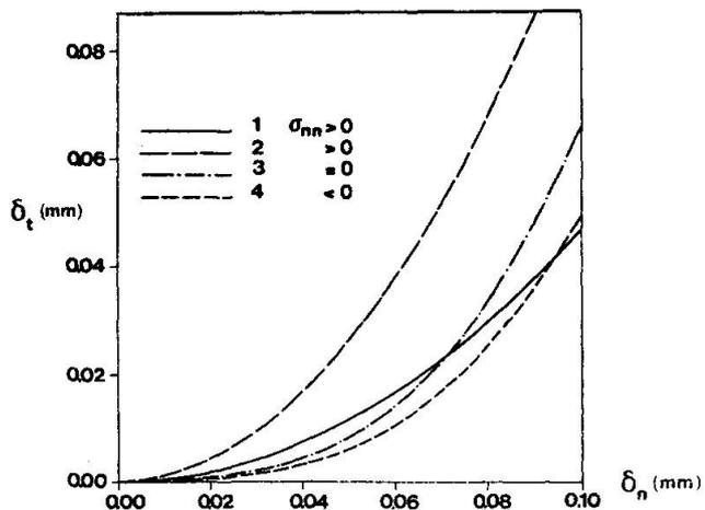
Fig.8 - Curves of the apparent shear modulus  $G^{CR}$  (tangent) for cracked reinforced concrete ( $f'_c = 31 \text{ N/mm}^2$ ,  $f_{sy} = 460 \text{ N/mm}^2$ ,  $p_x = p_y = 0.0112$ ,  $m = -1$ ,  $\alpha = 45^\circ$ ).
