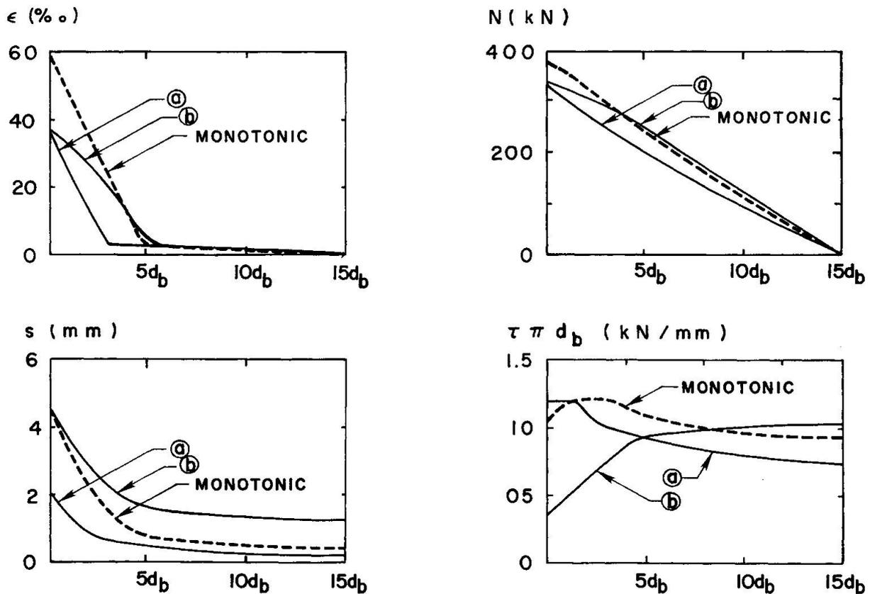
Fig. 9b Distribution of steel strain, slip, normal force and bond force along the bar at  $s = 2$  mm and  $s = 4.5$  mm for monotonic and cycling loading.
