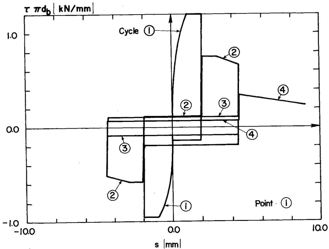
Fig. 9d Bond force-total slip relationship at loaded end.
