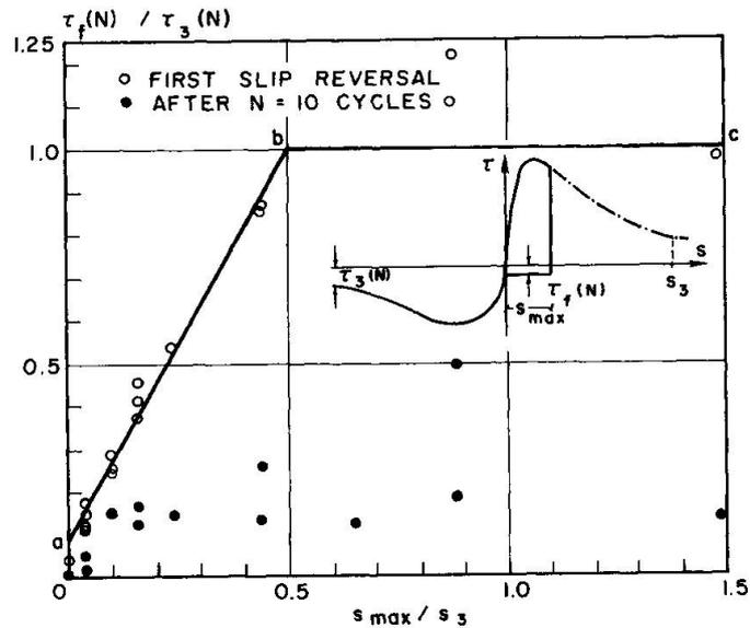
Fig. 7 Relationship between the frictional bond resistance  $\tau_f(N)$  and the corresponding ultimate frictional bond resistance  $\tau_3(N)$ .
