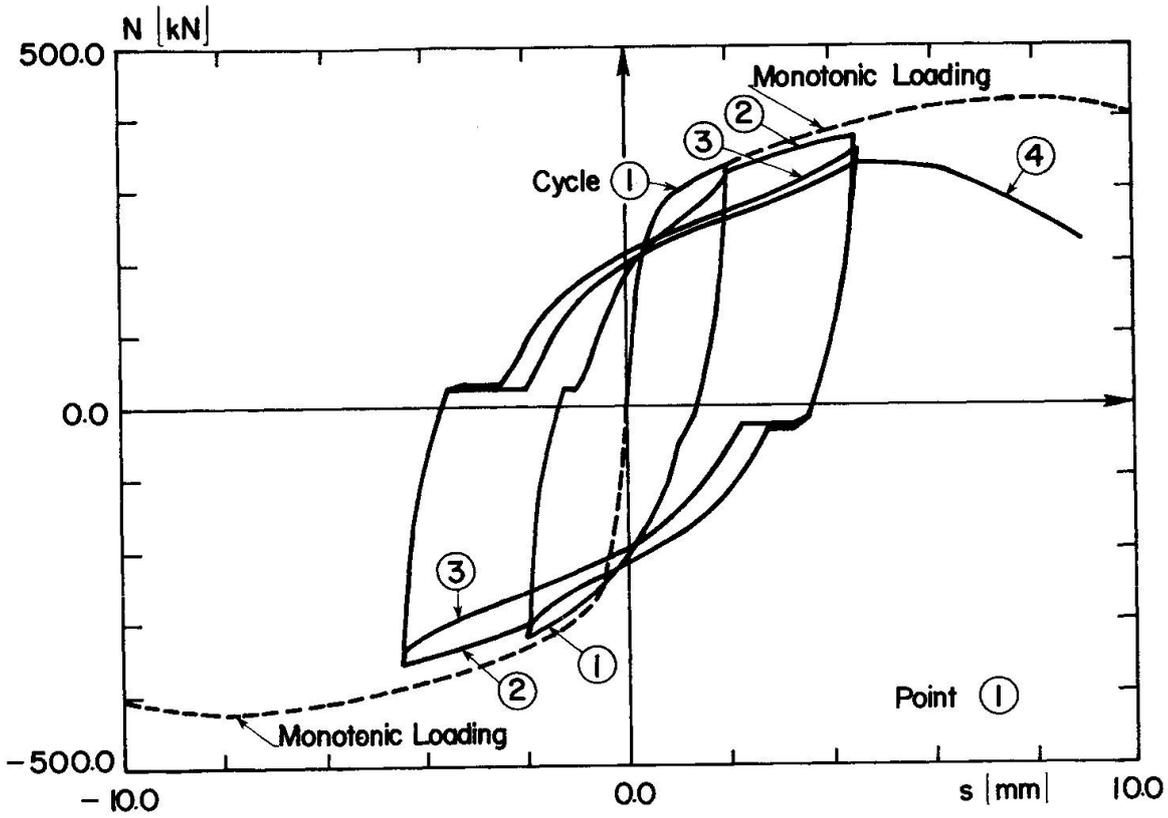
Fig. 9c Normal-force total slip relationship at loaded end.
