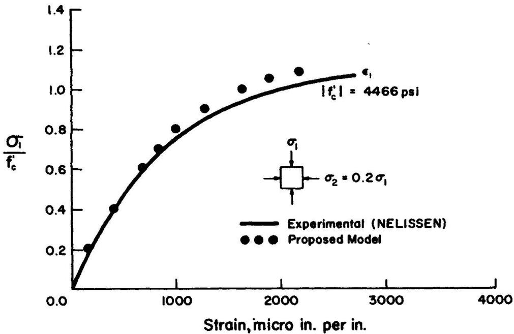
Fig. 13 Biaxial Compression of Plain Concrete,  $\sigma_2 = 0.2\sigma_1$
