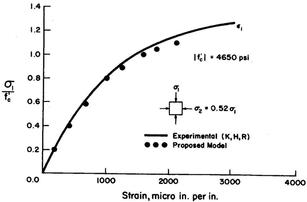
Fig. 15 Biaxial Compression of Plain Concrete,  $\sigma_2 = 0.52\sigma_1$
