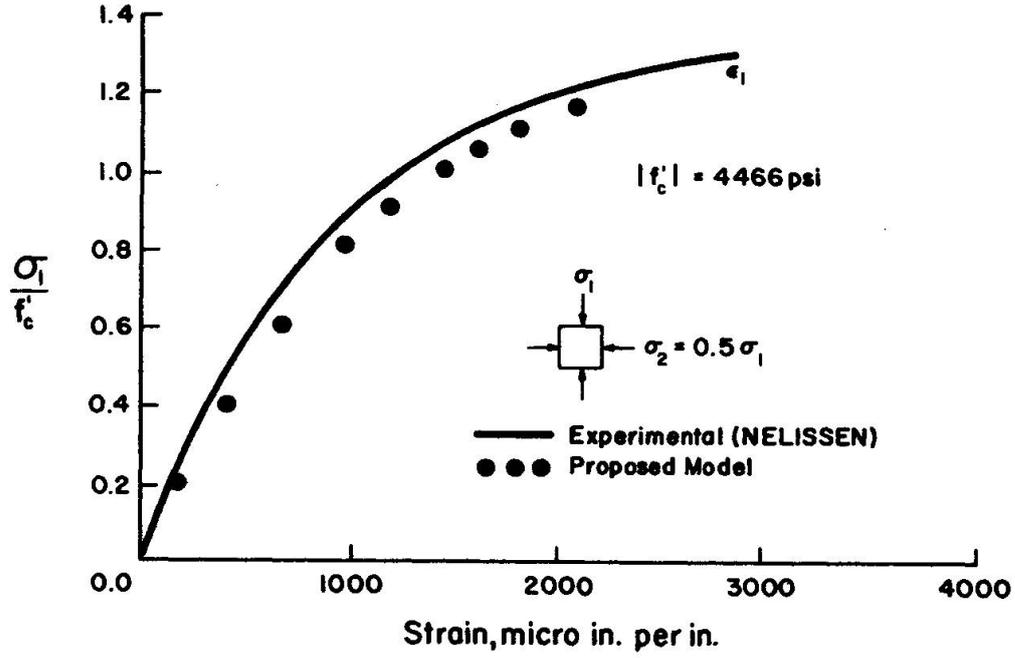
Fig. 14 Biaxial Compression of Plain Concrete,  $\sigma_2 = 0.5\sigma_1$
