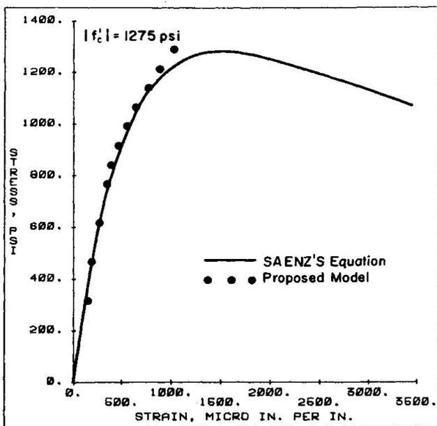
Fig. 9 Uniaxial Compression of Plain Concrete,  $|f'_c| = 1275$  psi
