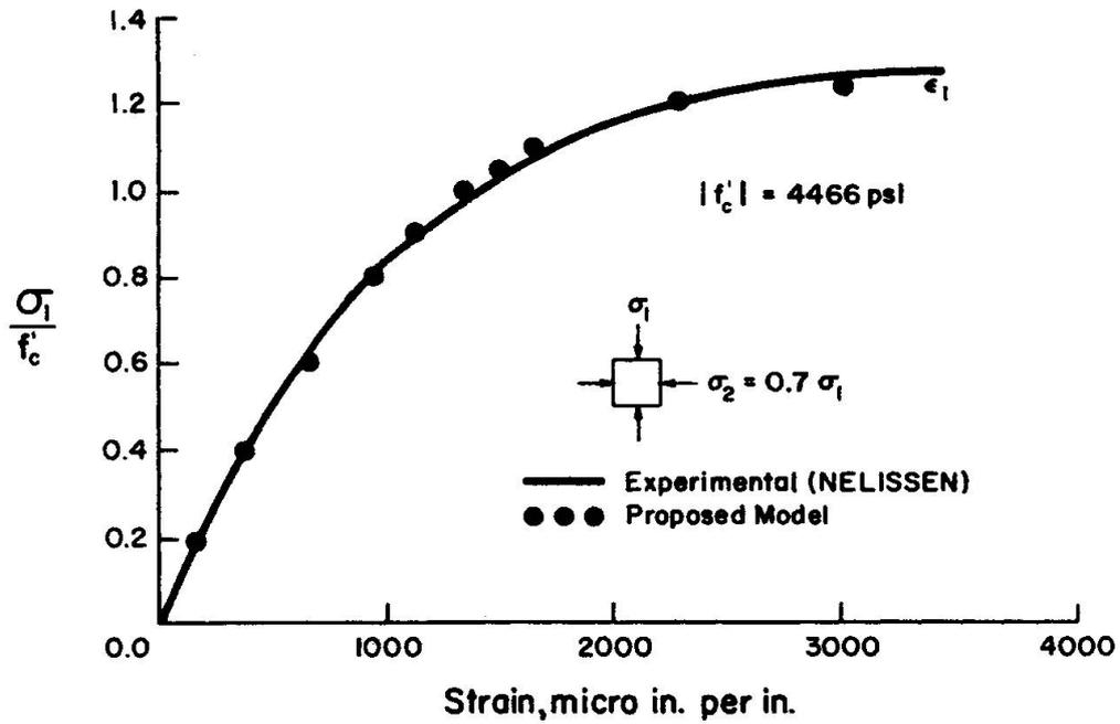
Fig. 16 Biaxial Compression of Plain Concrete,
