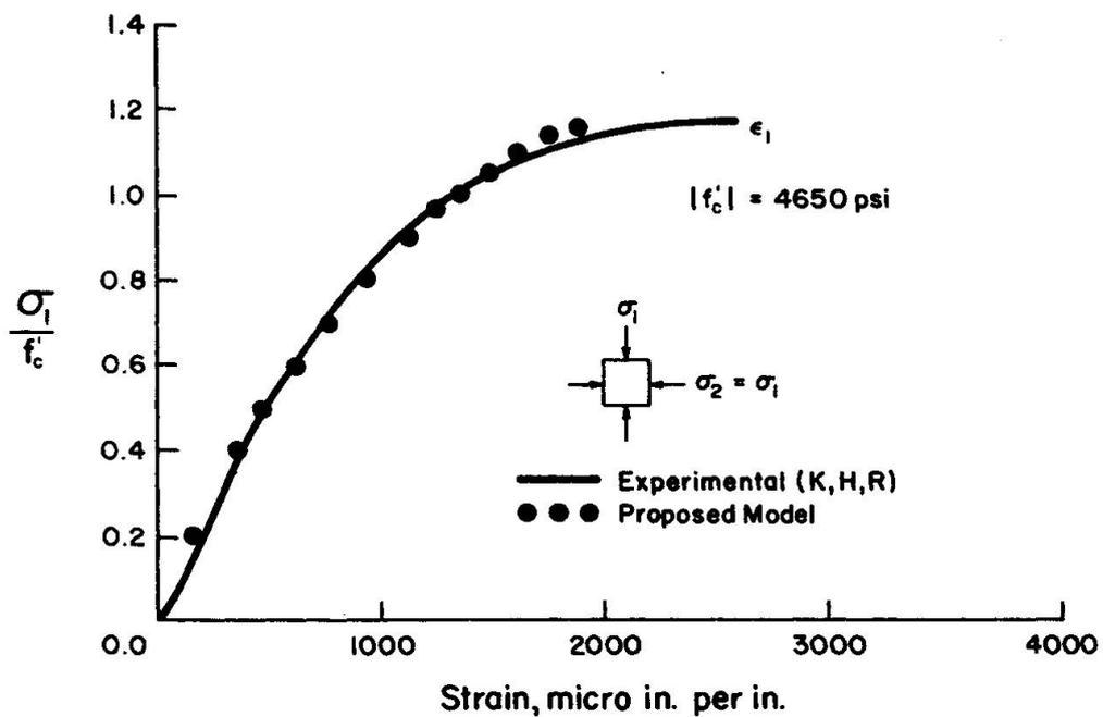
Fig. 17 Biaxial Compression of Plain Concrete,
