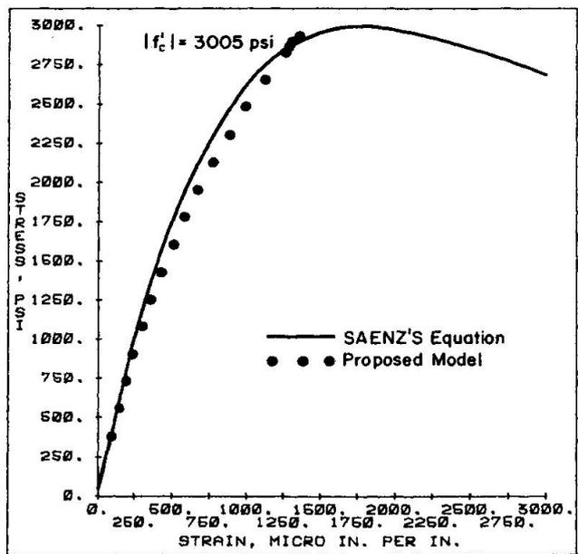
Fig. 10 Uniaxial Compression of Plain Concrete,  $|f'_c| = 3005$  psi
