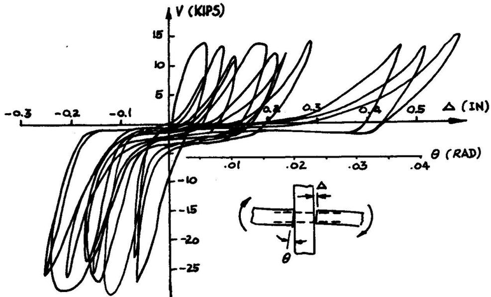
FIG. 3 SHEAR FORCE - BAR SLIP DIAGRAM (REF. 14)
