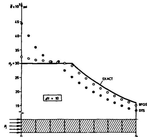
Fig. 11: EQUIVALENT STRESS DISTRIBUTION AT THE TIME  $t = 10$  sec
