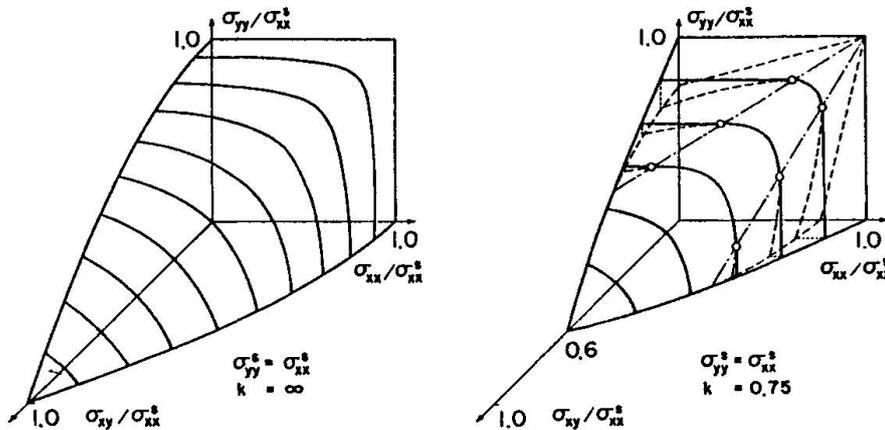
**Fig. 13** Example of Yield Surfaces of Net-Reinforced Panel [54,68]
