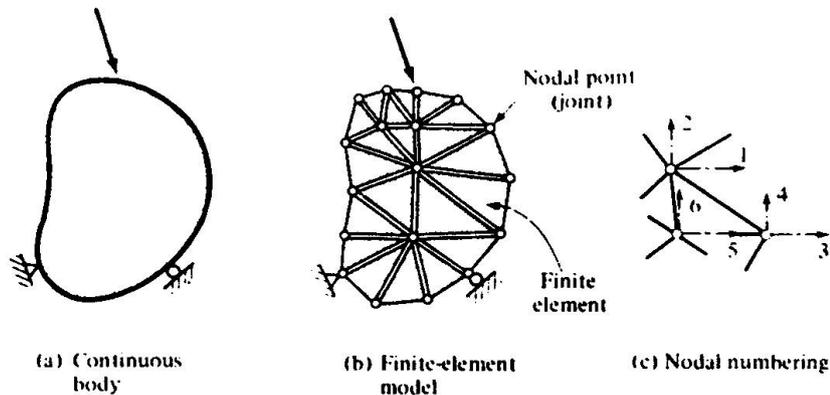
Fig. 1 Finite-element Model
