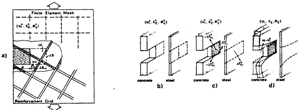
**Fig. 16** Crack Band Advance in Finite Element Mesh
