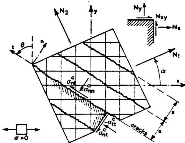
Fig. 11 Forces on the Cracks in Reinforced Concrete
