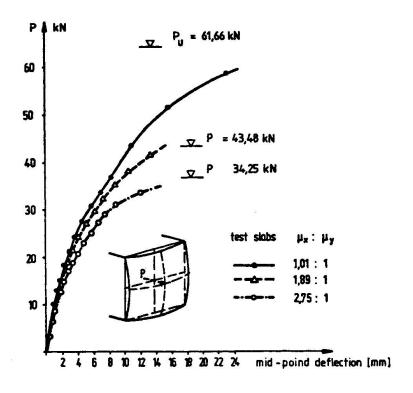
Fig. 3 Deflection Curves- Slab Tests [19]
