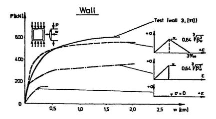
Fig. 5 Comparsion- Calculations with Different Assumtion for Tension- Stiffening [28]
