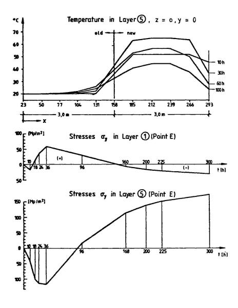
Fig. 13 Stresses in The Web of a Bridge- Girder Due to Hydration of Concrete [33]
