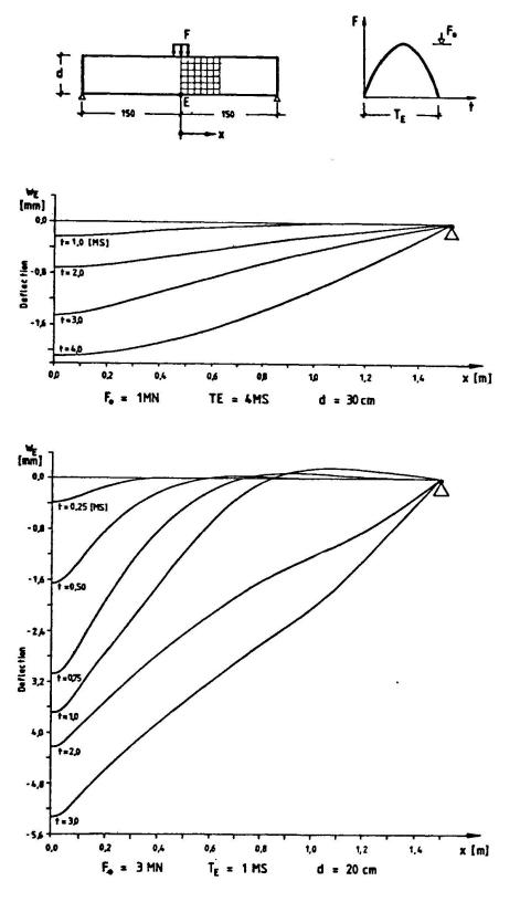
Fig. 12 Midpoint E- Deflection of Thick Slab Under Impact [26]
