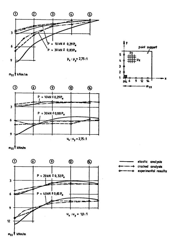
$\frac{\text{Fig. 4}}{\text{Axes of Symmetry [19]}}$  Experimental and Analytical Distribution of Moments  $m_{22}$  in
