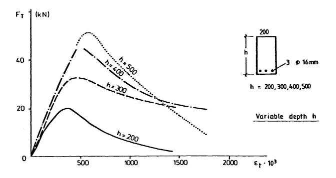
Fig. 7 Tension Force Versus  $\varepsilon_{t}$  According to Experiments [32]
