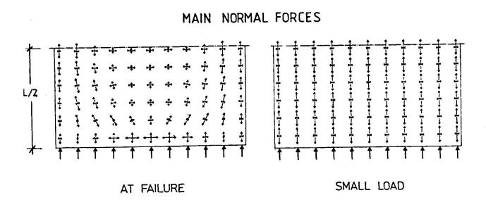
Fig. 6 Bearing Behaviour of RC- Walls Including Second Order Effects [28]
