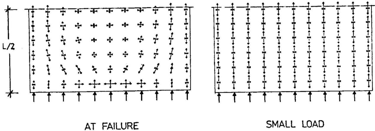
Fig. 6 Bearing Behaviour of RC- Walls Including Second Order Effects [28]
