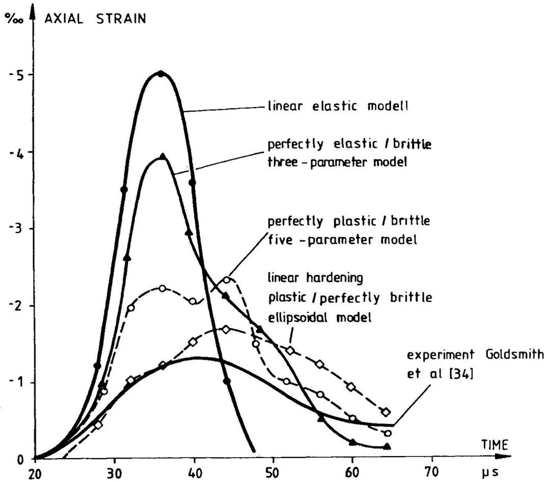
Fig. 11 Contact Problem- Different Constructive- Laws [25]
