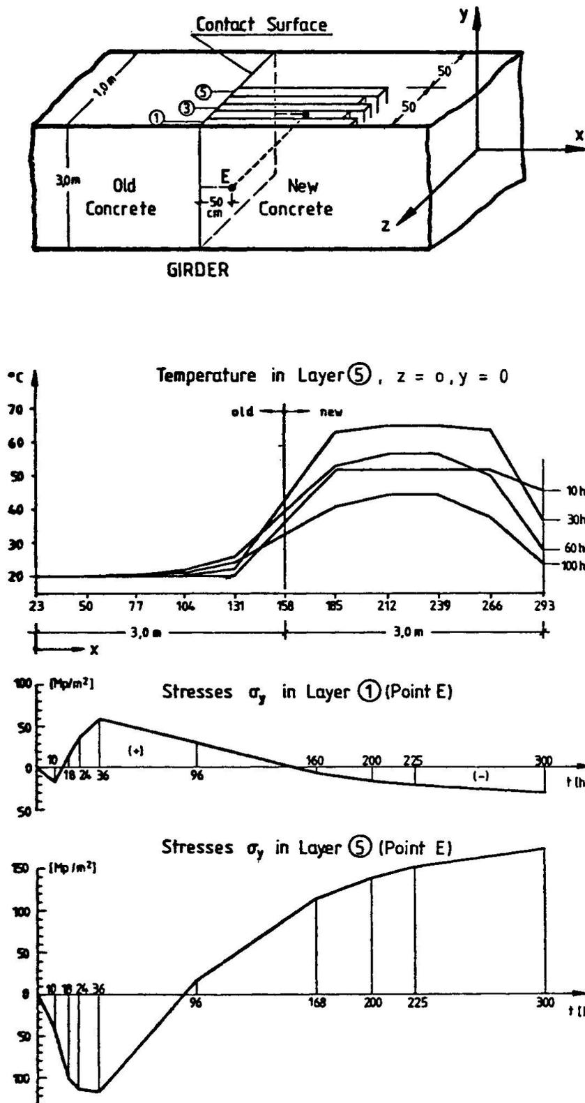
Fig. 13 Stresses in The Web of a Bridge- Girder Due to Hydration of Concrete [33]
