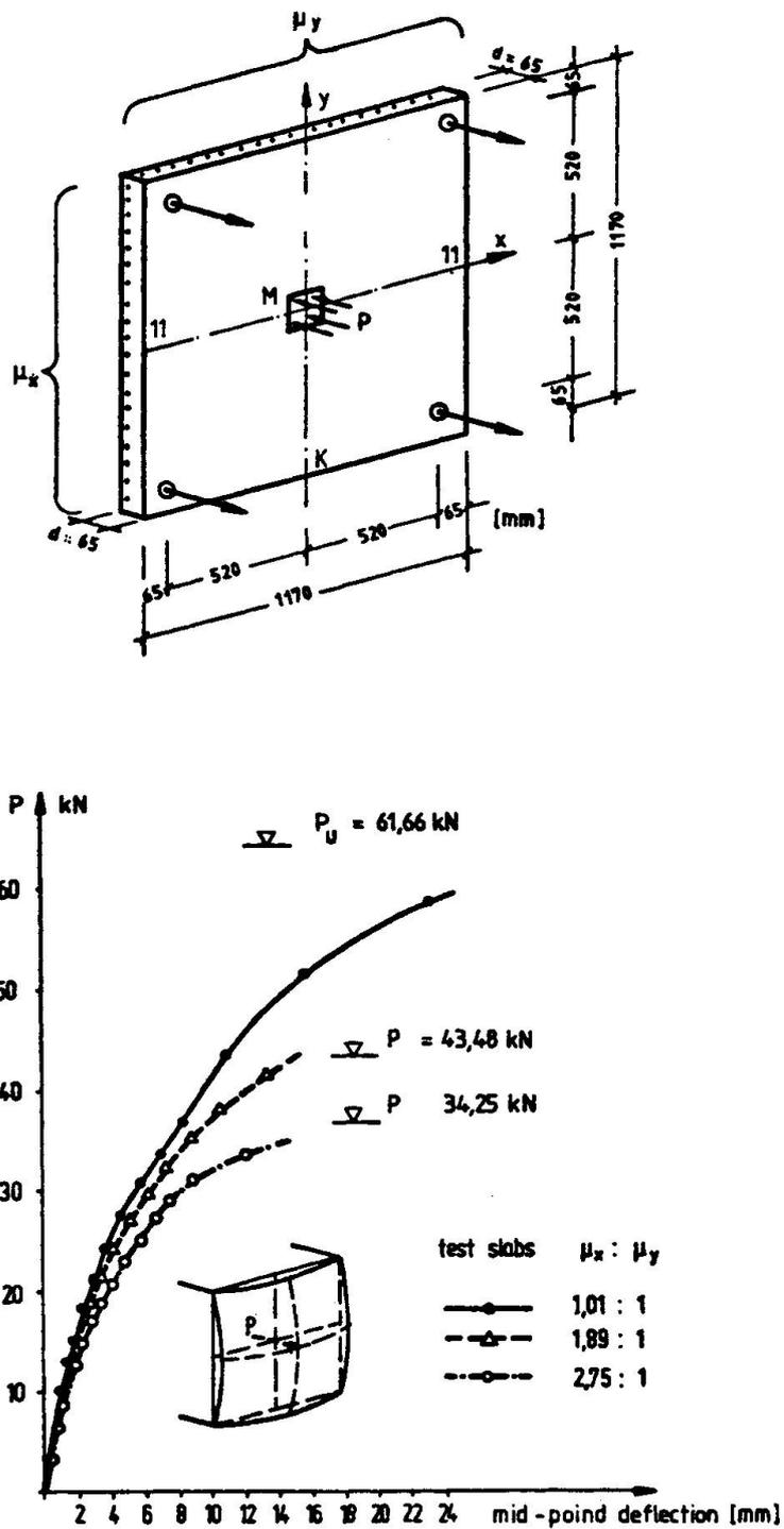
Fig. 3 Deflection Curves- Slab Tests [19]
