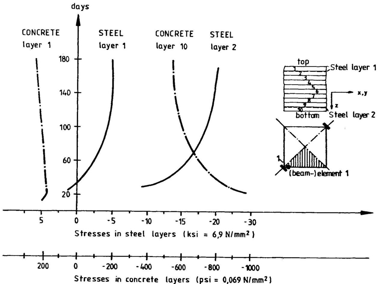
Fig. 10 Stresses Redistribution in Beam (Element 1)
