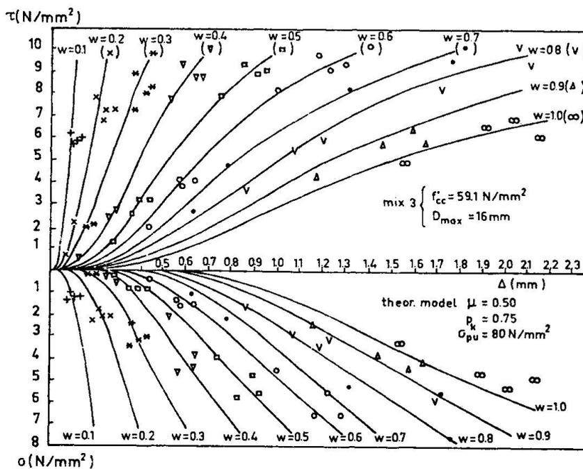
Fig. 5 Comparison Between Experimental Values for a Concrete with  $f'_{cc} = 59 \text{ N/mm}^2$  (8428 psi),  $D_{max} = 16 \text{ mm}$  (0.63 inch) and theoretical values, with  $p_k = 0.75$ ,  $\mu = 0.50$  and  $\sigma_{pu} = 80 \text{ N/mm}^2$  (11428 psi) ( $1 \text{ N/mm}^2 = 0.007 \text{ psi}$ ,  $1 \text{ mm} = 0.039 \text{ in.}$ )
