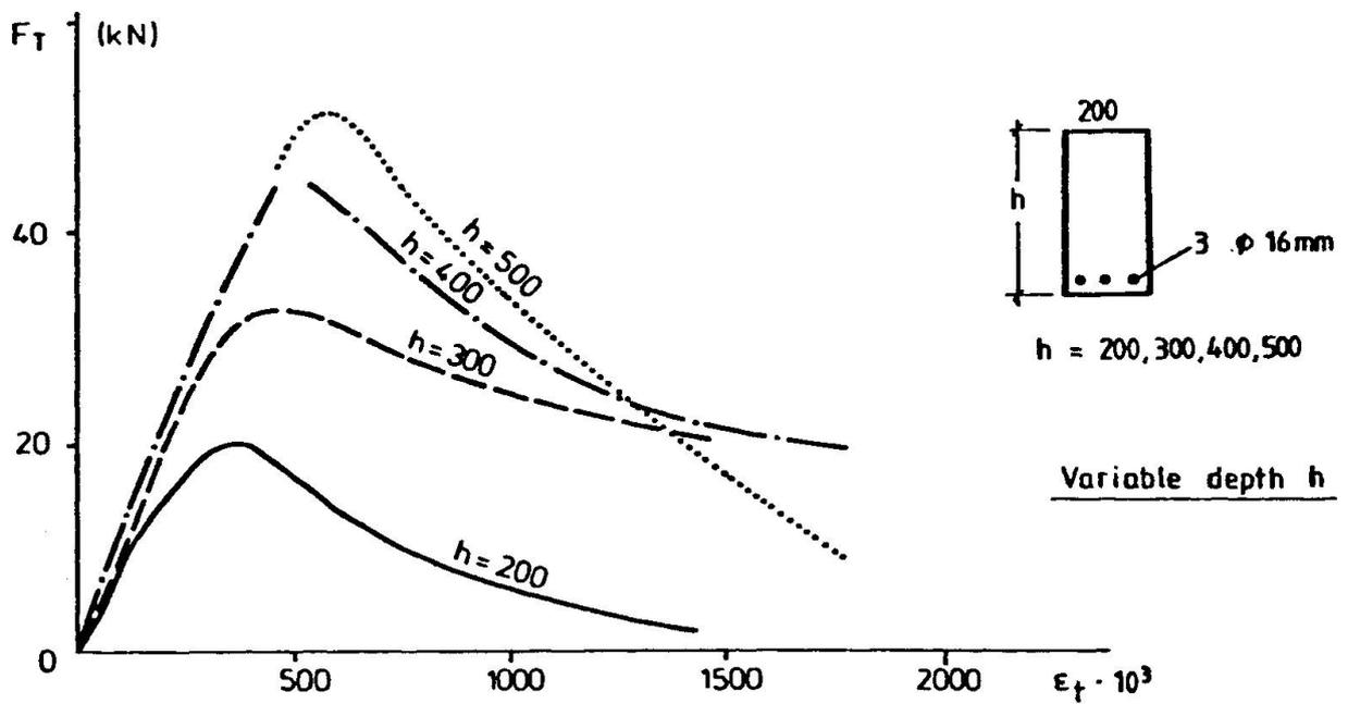
Fig. 7 Tension Force versus  $\epsilon_t$  According to Experiments [32]
