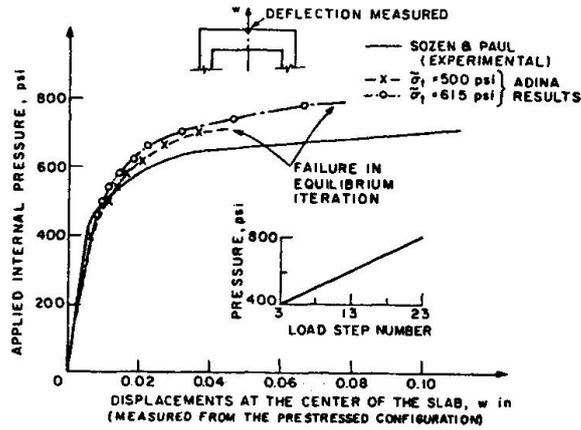
a. Displacements of the slab at mid-span
