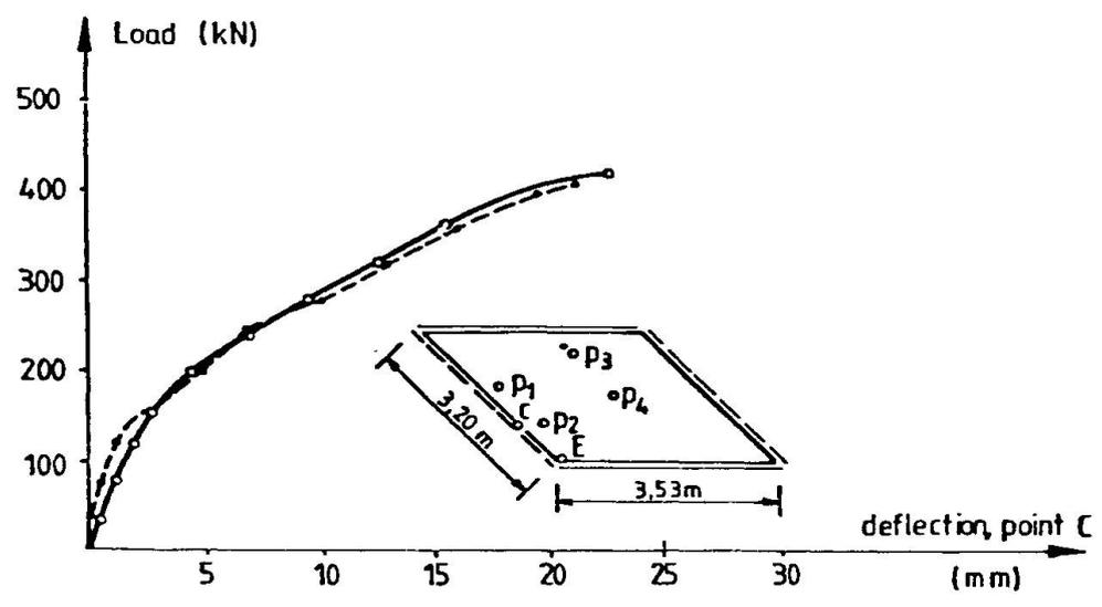
Fig. 8 Bearing Behaviour of Skew Slab [24]
