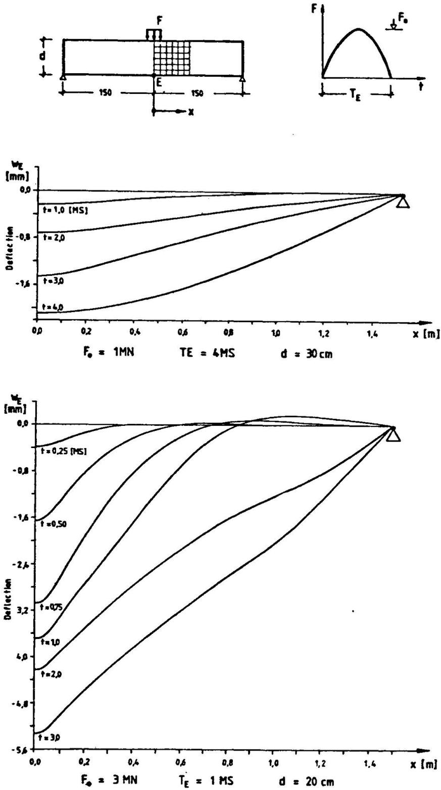
Fig. 12 Midpoint E- Deflection of Thick Slab Under Impact [26]
