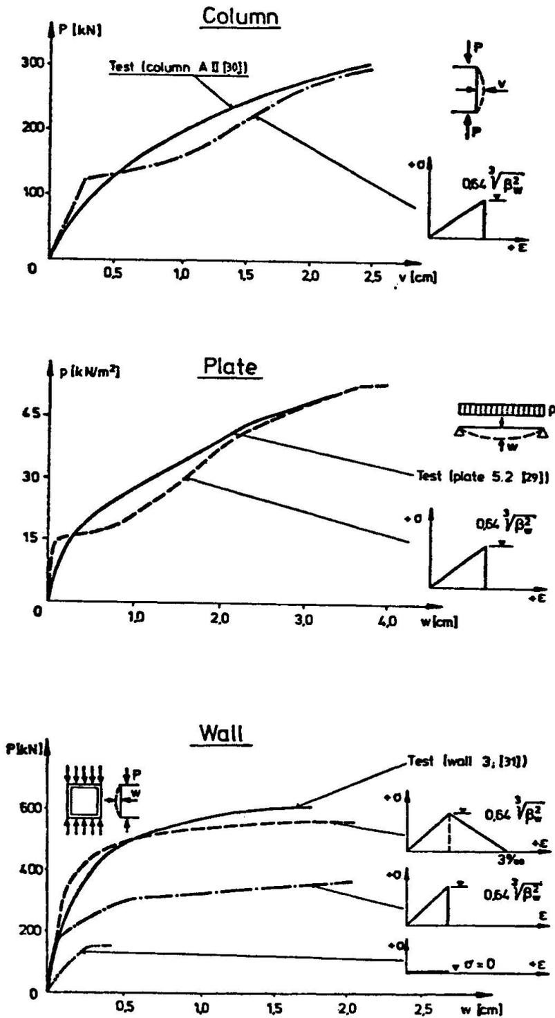
Fig. 5 Comparison- Calculations with Different Assumption for Tension- Stiffening [28]
