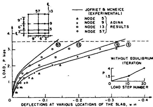
Fig. 17 Vertical Deflections of the Corner-Supported Concrete Slab
