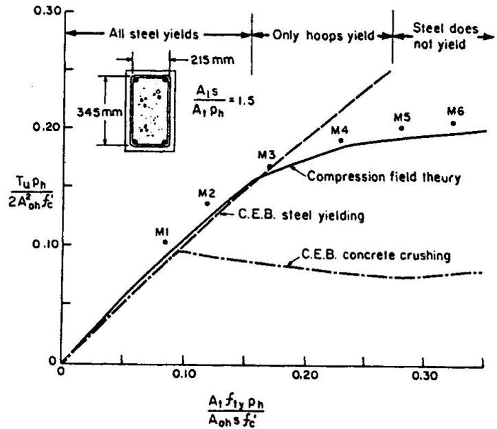
Fig. 8 Torsional Capacity versus Amount of Reinforcement
