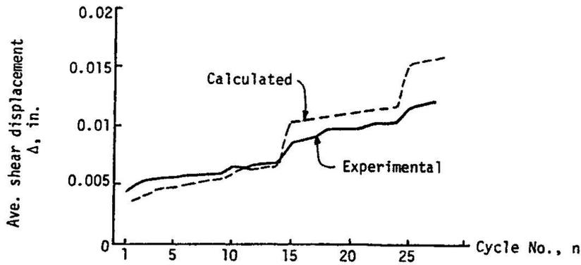
Fig. 6 Increase in Maximum Shear Displacement with Cycling
