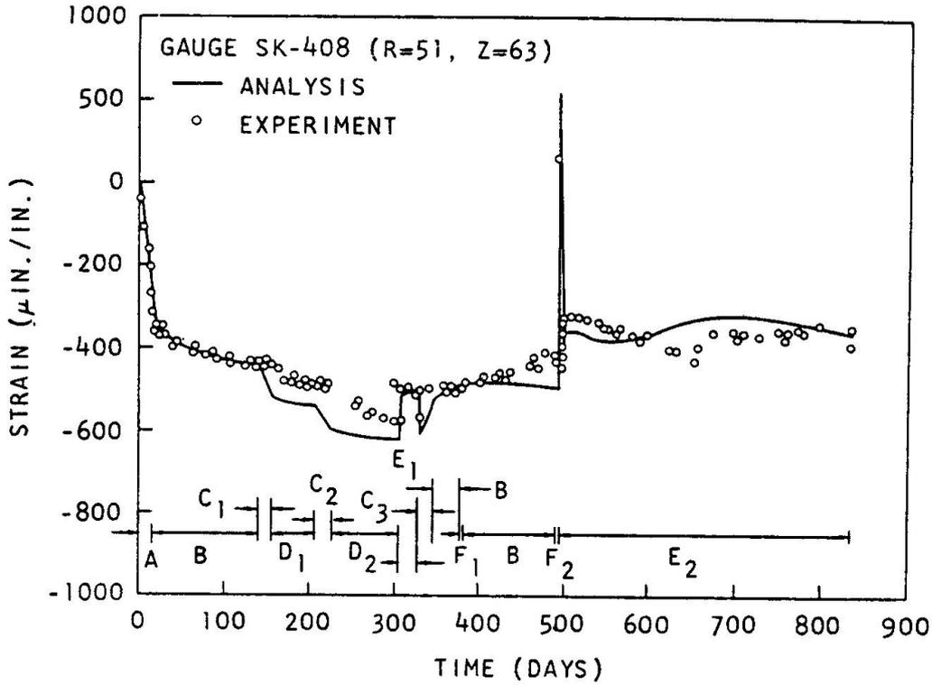
Fig. 15a Axial Concrete Strain at Haunch .
