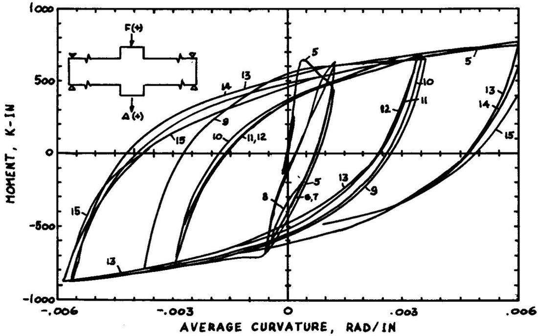
FIG. 1 MOMENT-CURVATURE DIAGRAM (REF. 10)
