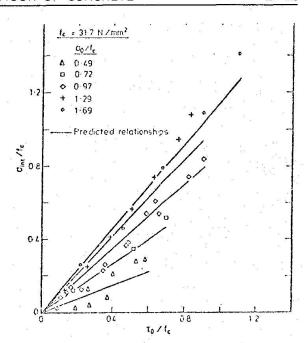
Fig. 4 Typical variation of oint with increasing applied stress
