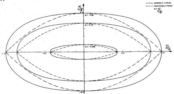
Fig.3 Yield Surfaces for Concrete Stress Resultants
