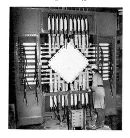
Fig. 11 New Test Rig for Shear Panels
