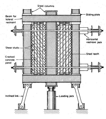
Fig. 3 Test Rig for Loading Panels in Shear
