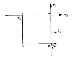
Fig. 2 Yield Criterion for Concrete
