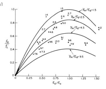
Fig. 10 Predicted and Observed Stress-Strain Relationships
