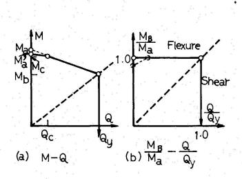
Fig. 5 Moment-Shear Force Interaction
