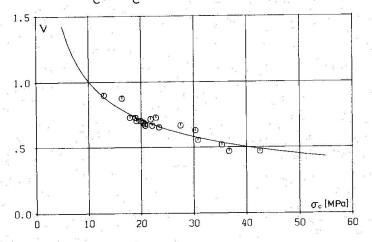
Fig. 4. Empirically determined  $\nu$ -curve:  $\nu = 3.2/\sqrt{\sigma}$ ,  $\sigma_c$  in MPa and test results from [79.1]
