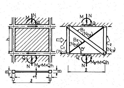
Fig. 1 Truss Model
