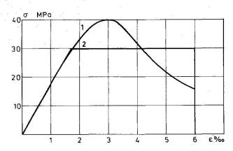
Fig. 2. 1:The analytical stress-strain curve.
