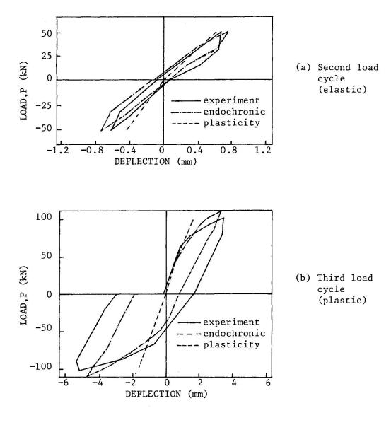
Fig.8 Results from analyses, Cervenka's shear panel
