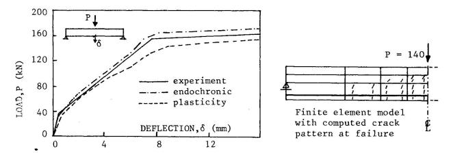
Fig.5 Results from analyses, Burns-Siess beam
