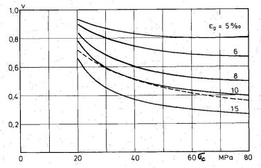
Fig. 3.  $\nu$  as a function of  $\epsilon$  and  $\sigma_c$ . The dashed curve g is the curve  $\nu = 3.2/\sqrt{\sigma}_c$ ,  $\sigma_c$  in MPa from fig.4.
