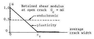
Fig.3 Shear retention factor
