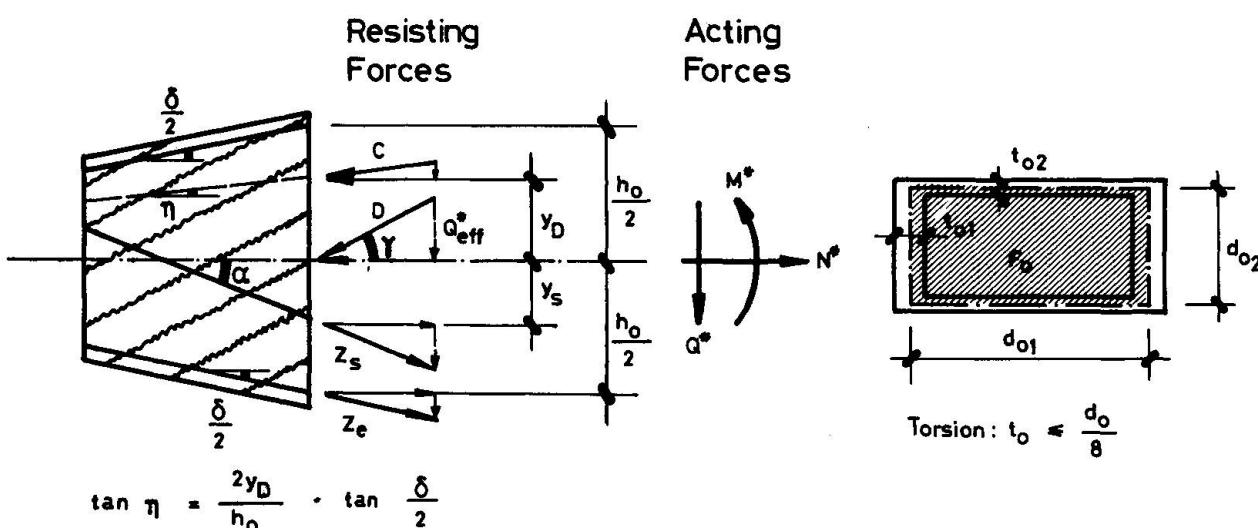
Fig. 3 Variable Depth and Inclined Tendons
