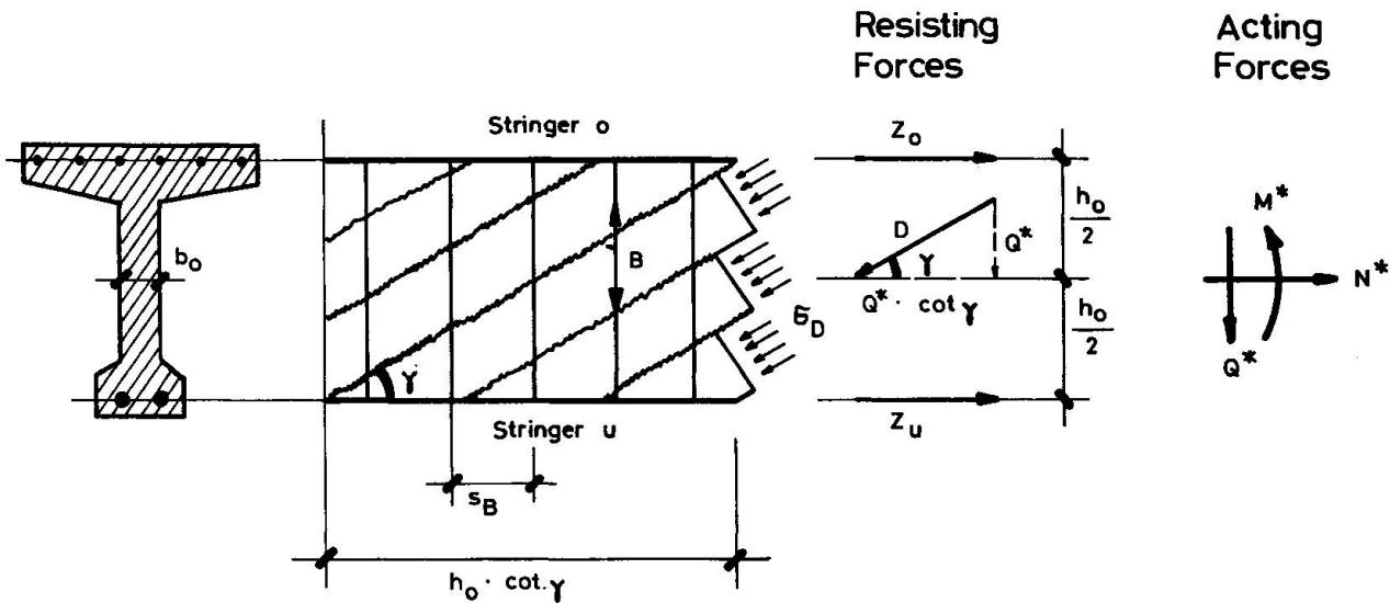
Fig. 1 Truss Model
