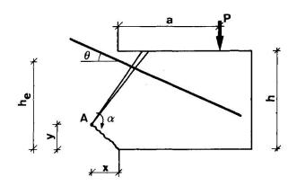
Fig. 7. Failure mechanism.
