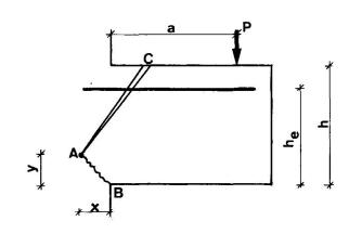
Fig. 5. Failure mechanism.
