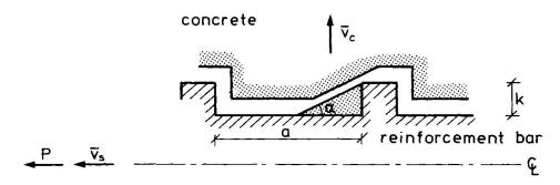
Figure 3: The Local Failure Mechanism
