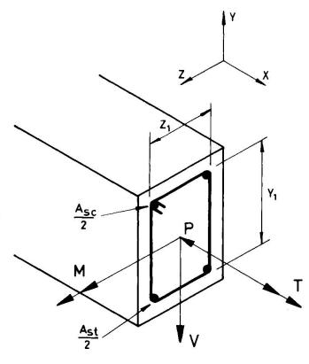
Figure 2. Rectangular Section and Loading
