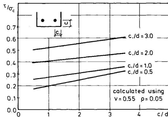
Figure 18: Calculated Strength  $\tau/\sigma_c$  as a Function of the Covers  $c$  and  $c_1$ .
