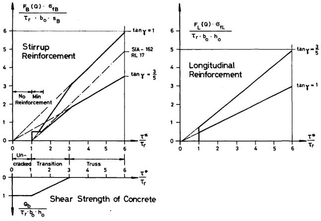
Fig. 2 Design of Shear Reinforcement
