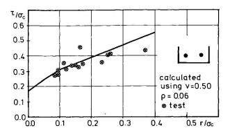
TIOC 0.6 the main bar 0.5 is yielding 0.4 0.3 calculated 0,2 using v=0.50p = 0.060.1 **⊗** test 0.0 0.4 0.5 r/σ<sub>c</sub> 0.0 0.1 0.2 0.3
