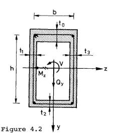
If  $M_z > \frac{1}{2} V (h+b)/b$  the longitudinal reinforcement in the top flange can be chosen to be zero, while the force in the longitudinal reinforcement in the bottom flange still has to be increased by  $M_z/h$ .
