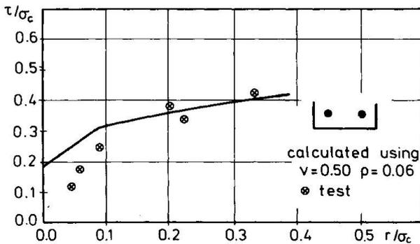
Figure 15: Tentor-steel 56  $\phi 14$ . Comparison between Tests and Calculations.
