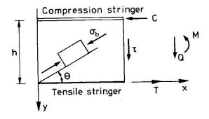
The necessary reinforcement in the x- and the y-direction and the concrete stress  $\sigma_b$  is determined by (1.11)-(1.13). We find
