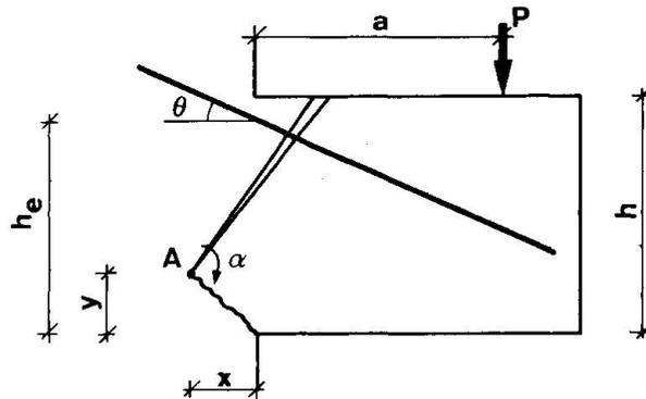
Fig. 7. Failure mechanism.
