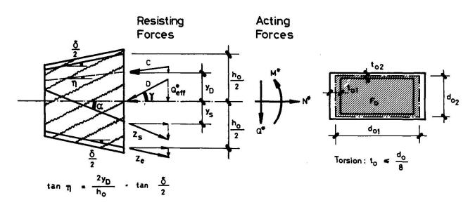
Fig. 3 Variable Depth and Inclined Tendons
