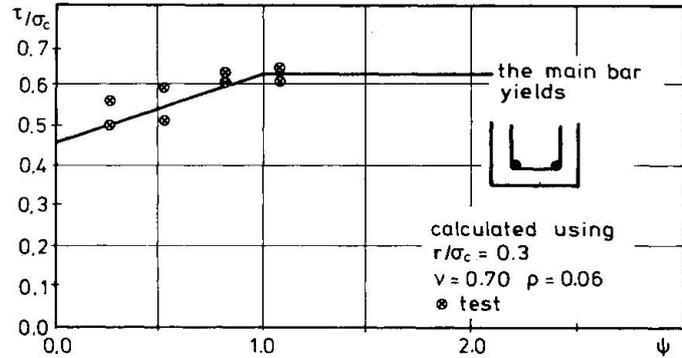
Figure 16: Comparison between Tests and Calculations of the Anchoring of Kamsteel 42  $\phi 14$  with Stirrups at the Supports.
