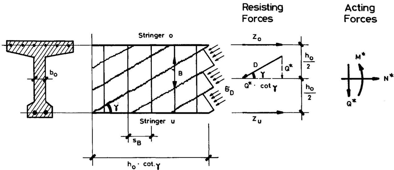
Fig. 1 Truss Model
