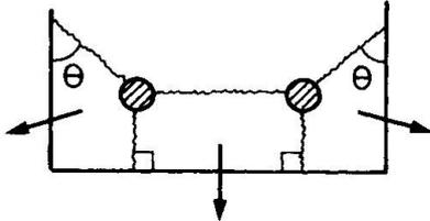
Figure 10: Failure 2, the Cover Splits into Three Pieces.
