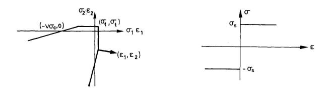
Figure 1: Modified Coulomb Failure Cri- Figure 2: Rigid-plastic Stress-strain terion for plane strain with the Associated Flow Rule. Reinforcement.
