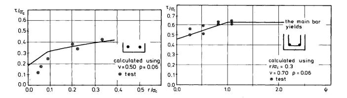
Figure 15: Tentor-steel 56 Ø14. Compa- Figure 16: rison between Tests and Calculations.
