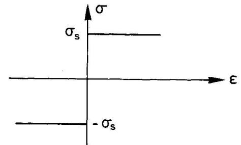
Figure 1: Modified Coulomb Failure Criterion for plane strain with the Associated Flow Rule.
