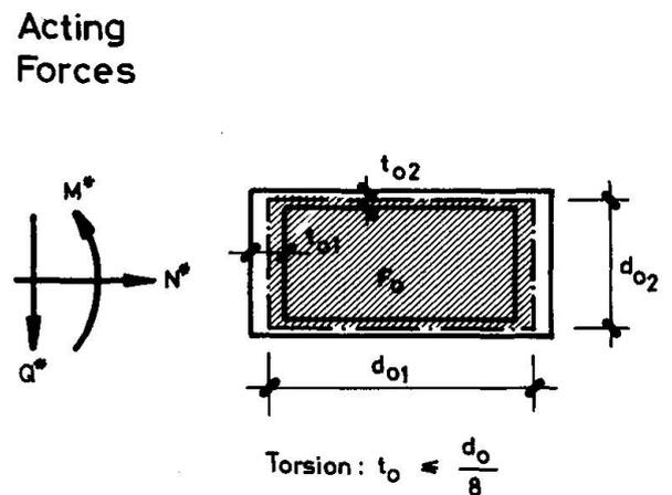
Fig. 4 Effective Wall Thickness for Torsion
