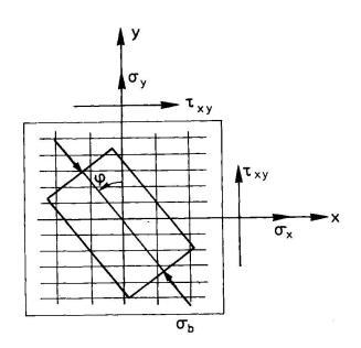
If for some reason the reinforcement in one direction is known, or if the optimum value of the total reinforcement of the structure is found for other inclinations of the compressive stresses than found above, see section 2, the following formulas determine the necessary amount of reinforcement:
