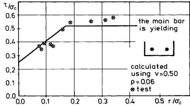
Figure 14: Kamsteel 42  $\phi 10$ . Comparison between Tests and Calculations.
