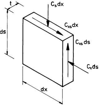
Figure 1. Concrete Sheet Element
