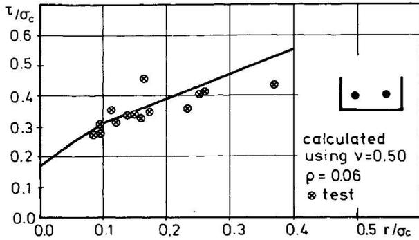
Figure 13: Kamsteel 42  $\phi 14$ . Comparison between Tests and Calculations.
