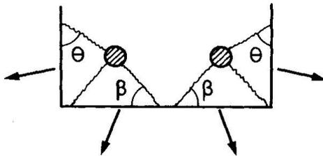
Figure 11: Failure 3, the Corners Split into Two Pieces
