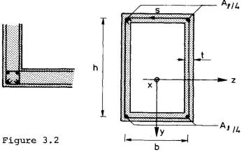
If the yield stresses in both reinforcement directions are equal to  $\sigma_{\text{f}}$ , we get by means of (1.1) and (1.2) the following reinforcement areas per unit length:
