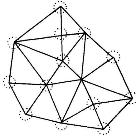
For example, the complementary solution total normal bending moments at the FE sides of the mesh represented in Fig. 3 may be expressed in terms of two static parameters ( $p_1$  and  $p_2$ ) in the following form
