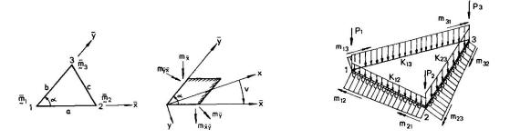
Fig. 3.2 Triangular element, TRIL. Fig. 3.3 Boundary forces.
