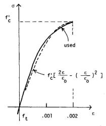
FIG.1 STIFFNESS OF CONCRETE
