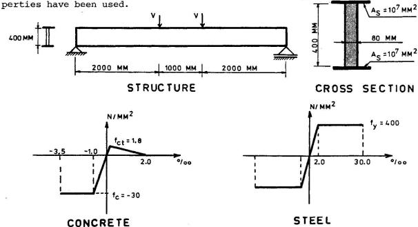
Survey of the structure that was investigated and Fig. 5 the stress-strain relations used for a unit web effectiveness factor.
