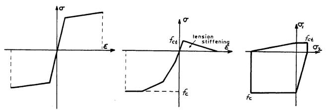
Fig. 3 Possible stress-strain relation for steel
