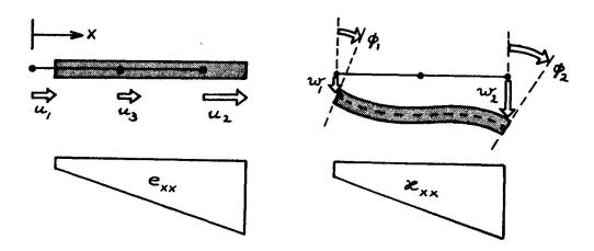
Fig. 1 Degrees of freedom and deformations for axial strain  $e_{\mathbf{X}\mathbf{X}}$  and curvature  $\kappa_{\mathbf{X}\mathbf{X}}$
