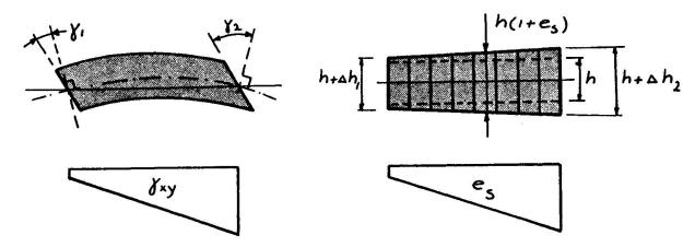
Fig. 2 Extra degrees of freedom and deformations for shear  $\gamma_{\rm XV}$  and vertical strain  $e_{\rm S}$
