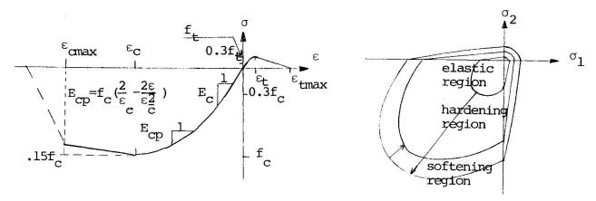
Fig. 1. Uniaxial stress-strain curve of concrete
