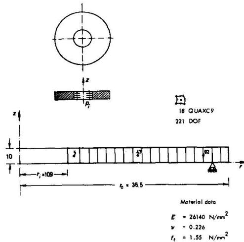
**FIG. 1** Configuration and axisymmetric idealisation
