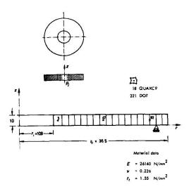
FIG. 1 Configuration and axissymmetric idealisation
