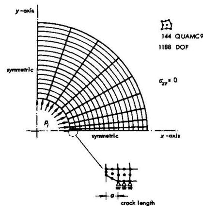
**FIG. 4** Plane stress idealisation of discrete crack
