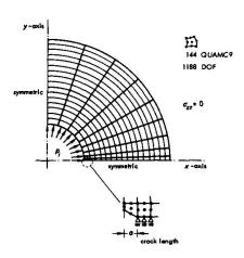
FIG. 4 Plane stress idealisation of discrete crack
