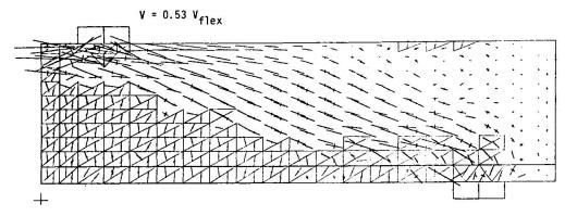
FIG.5 BEAM WITH CRACKING ALLOWED FOR ALL ELEMENTS
