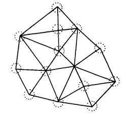
For example, the complementary solution total normal bending moments at the FE sides of the mesh represented in Fig. 3 may be expressed in terms of two static parameters ( $p_1$  and  $p_2$ ) in the following form
