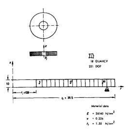
FIG. 1 Configuration and axissymmetric idealisation
