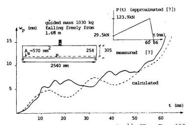
Fig. 3. Midspan deflection vs. time of RC beam, E = 44 GPa, E = 100 MPa, f = 60 MPa, f = 6 MPa, v=0.2, p=.24E-8Ns/mm<sup>2</sup>, E = 210 GPa, E = 1 GPa, f = 520 MPa, v=0.3, 5 elements for half span, time integration by trapezoidal rule.
