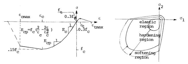
Fig. 1. Uniaxial stress-strain curve of concrete
