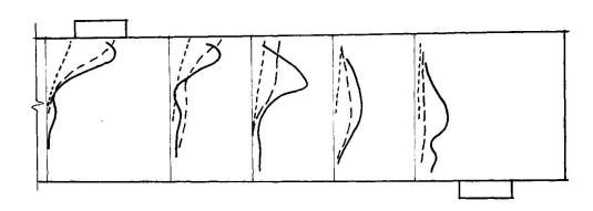
FIG.6 PREDICTED DISTRIBUTION OF COMPRESSIVE PRINCIPAL STRESSES FOR SHEAR 0.18, 0.44 AND 0.53  $V_{\mbox{flex}}$
