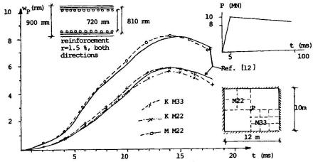
Fig. 4. Deflection vs. time of rectangular plate under central jet force. E = 210 GPa, E = 33 GPa, v=0.15, f = 22.7 MPa, f = 2.27 MPa, f = 400 MPa,  $\rho$ =0.24E-8 Ns /mm ,  $\epsilon$  = 0.002,  $\epsilon$  = 0.004,  $\epsilon$  = 0.0002, K = Kirchhoff plate theory, M = Mindlin plate theory.
