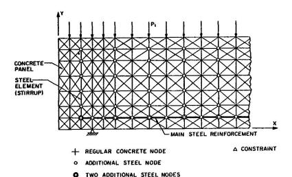
Figure 1. Finite element assemblage of a singly reinforced beam
