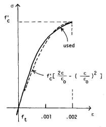
FIG.1 STIFFNESS OF CONCRETE
