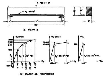
Figure 27. Example Problem 2: Simple Beam Loaded at Midspan
