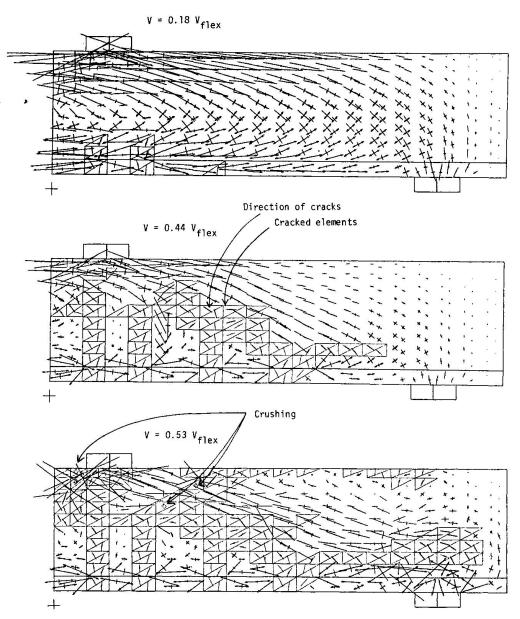
FIG. 4 PREDICTED PRINCIPAL STRESSES, CRACKING AND CRUSHING
