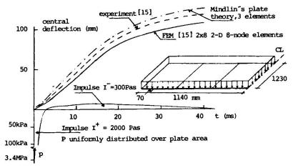
Fig. 5. One way roller supported slab under uniform pressure varying with time. Central deflection vs. time.
