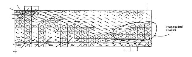
FIG.7 PREDICTED PROGRESSIVE PROPAGATION OF CRACKS ALONG REINFORCING BARS AT A SHEAR 0.44 V<sub>flex</sub>
