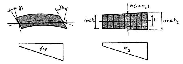
Fig. 2 Extra degrees of freedom and deformations for shear  $\gamma_{\rm XY}$  and vertical strain  ${\rm e_s}$
