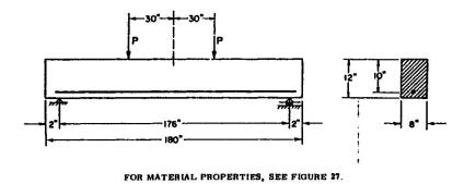
Figure 30. Example Problem 3: Simple Beam Loaded Symmetrically by
