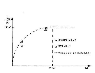
Fig. 8 Comparison of the ultimate strength from Stanil/1 and experiment.
