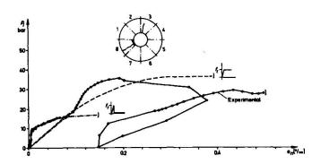
FIG. 2 Comparison of numerical and experimental results at the inside of sector 8
