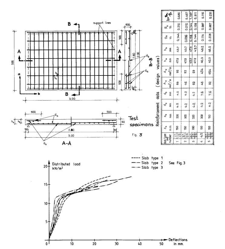
Fig. 4. Deformations of Slabs
