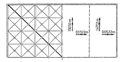
Fig. 3 Rectangular Slab with Free Edge - Optimal Solution for Two Bottom Reinforcing Grids
