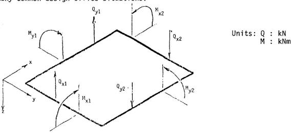
Fig. 2 Stress-Resultants on a Large Element
