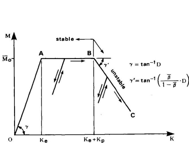
Fig. 1 Idealized Moment-curvature Curve.
