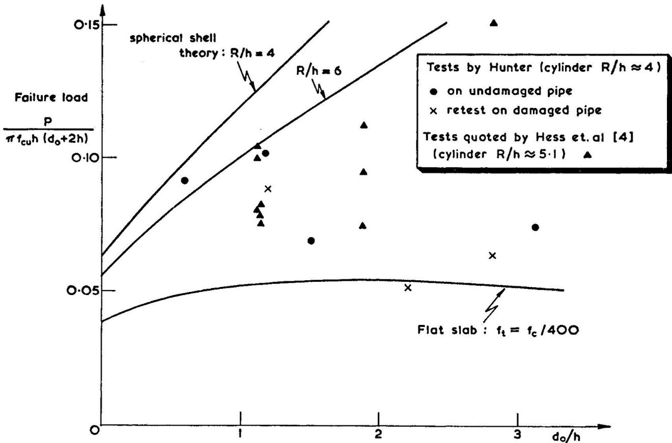
Fig. 5 Experimental results on cylinders in punching shear.
