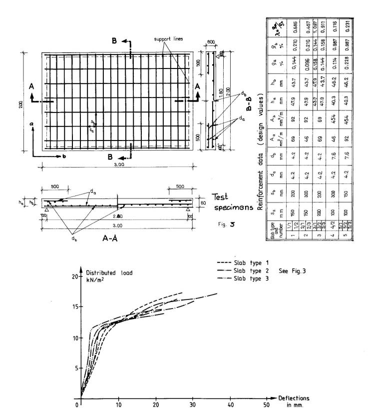
Fig. 4. Deformations of Slabs
