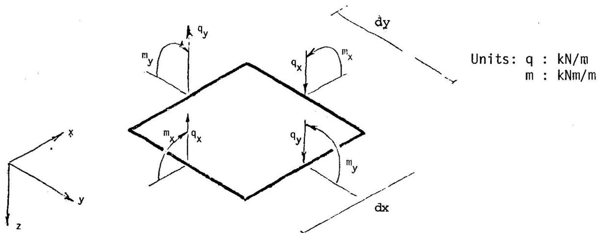
Fig. 1 Local Distributed Stress-Resultants on a Small Element
