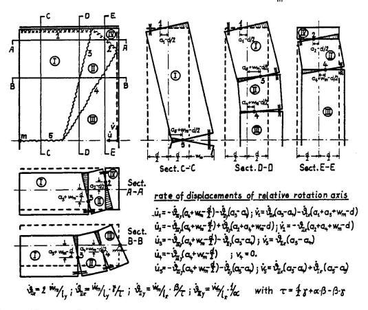
Fig. 4 Failure Mechanism in the Elevation
