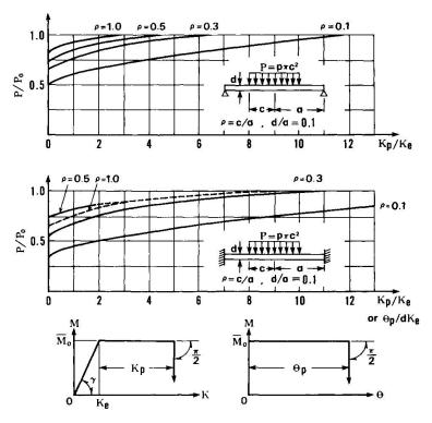
Fig. 4 Relationships Between Ultimate Loads and Limit Plastic Curvature or Limit Plastic Rotation.
