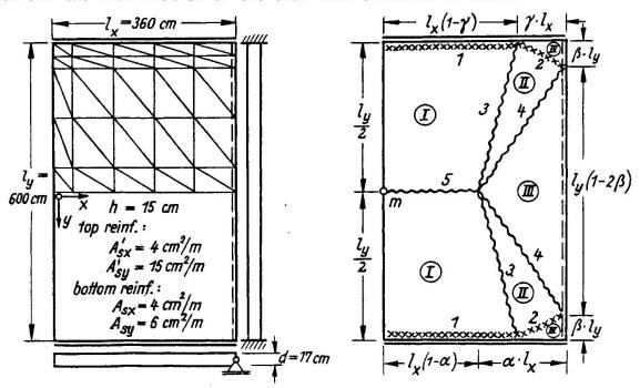
Fig. 1 System and Finite Element Idealization
