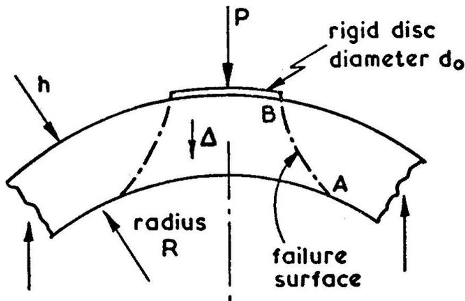
Fig. 1 A punching shear failure.
