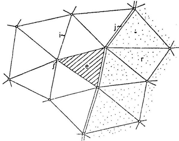
Fig. 1 Finite-element Mesh
