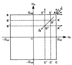
Fig. 2 Loading Surfaces.
