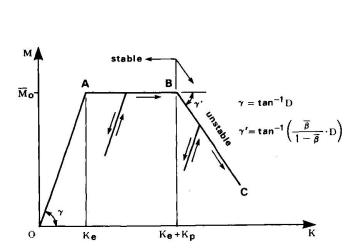
Fig. 1 Idealized Moment-curvature Curve.
