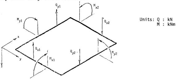
Fig. 2 Stress-Resultants on a Large Element
