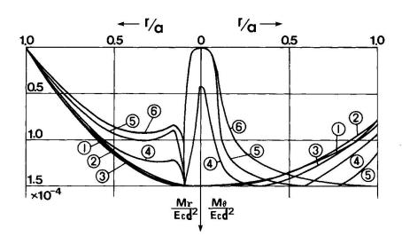
Fig. 7 Variations of Bending Moments along the Radius for the Simply Supported and Uniformly Loaded Slab with  $\bar{\alpha}$  = 0.25 and  $\bar{\beta}$  = 0.1 in Fig. 5.
