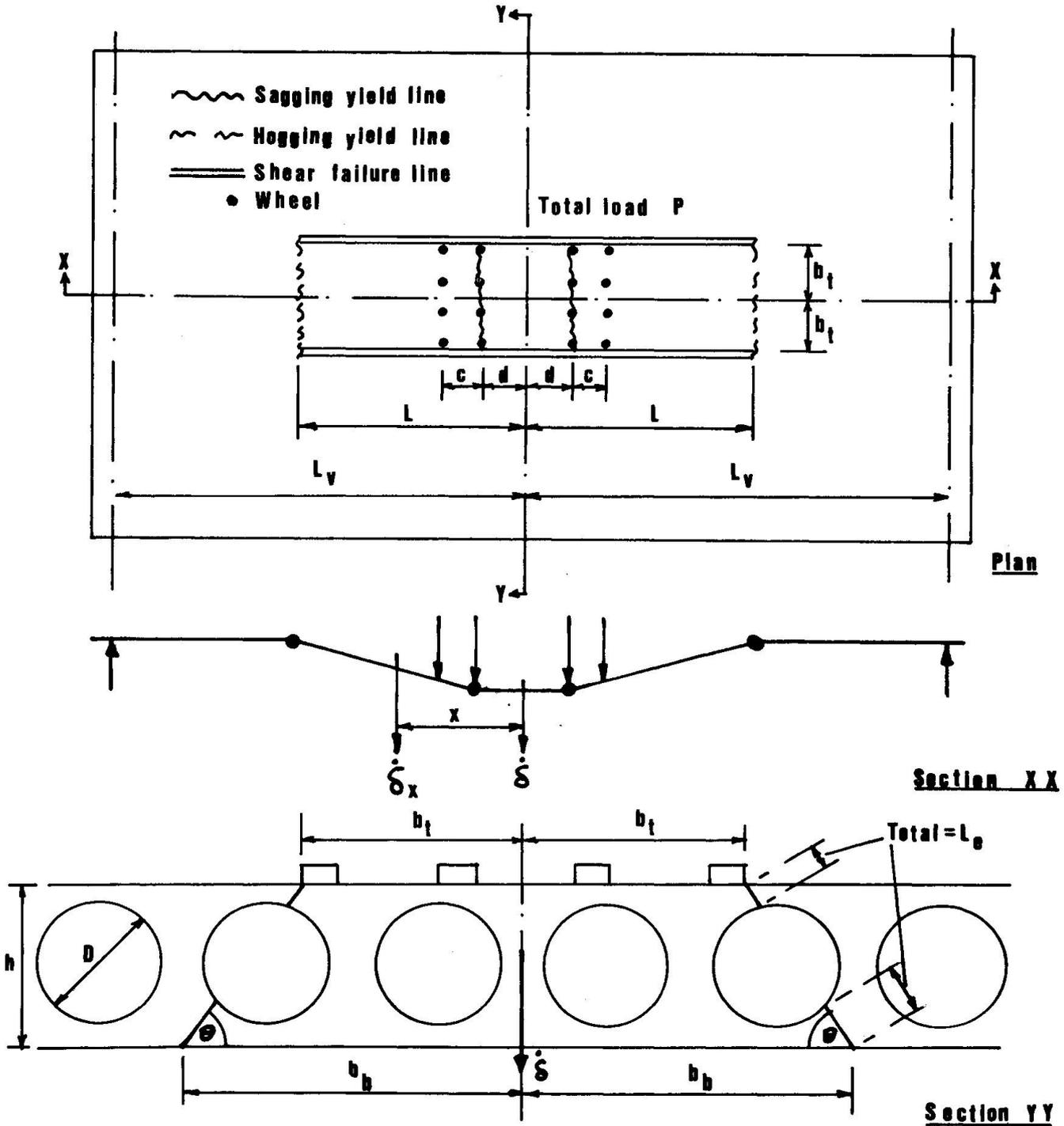
Fig. 1 Initial collapse mechanism
