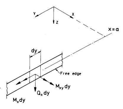
Figure 1. Apparent vanishing forces at free edge.
