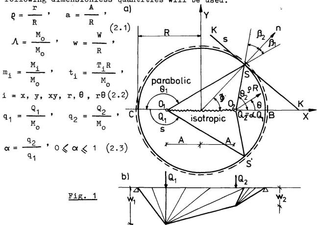
where W,  $\rm M_i$ , T, denote the deflection velocity, the bending moments and the shear forces respectively whereas R stands for the reference length which equals to the plate radius.
