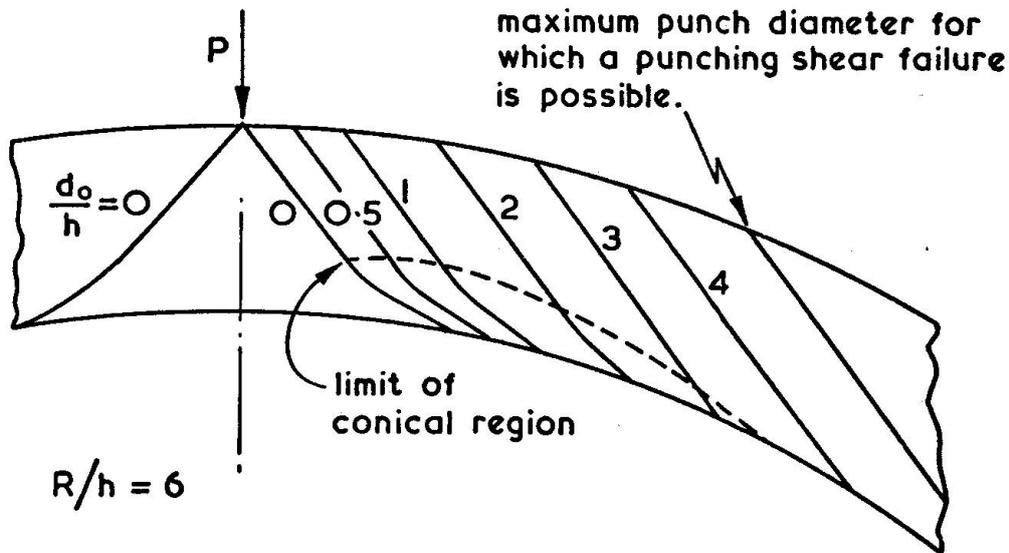
Fig. 3 Optimising curves for various punch diameters.
