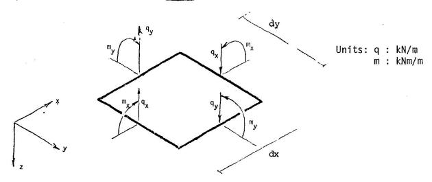
Fig. 1 Local Distributed Stress-Resultants on a <a href="Small Element">Small</a> Element
