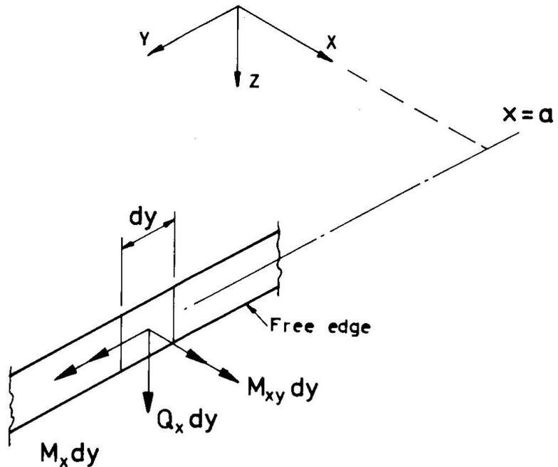
Figure 1. Apparent vanishing forces at free edge.
