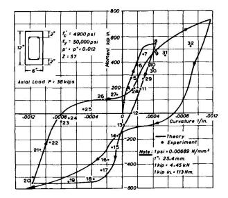
Fig. 2 Predicted Moment-Curvature Response Under Reversed Cyclic Loading [2]
