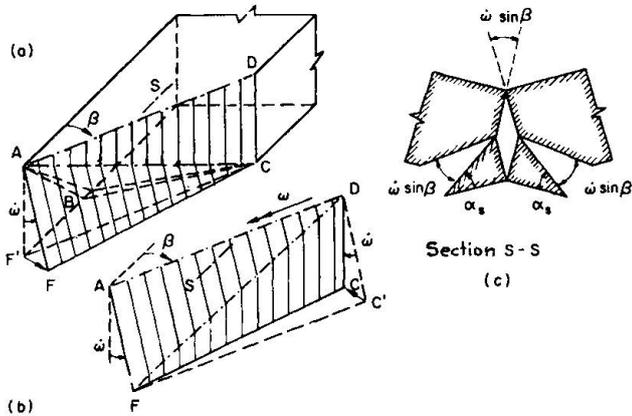
Fig. 6 Basic Torsional Mechanism for Solid Beams
