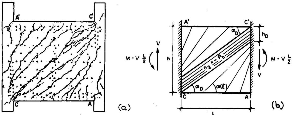
Fig. 9 Test Specimen of Deep Beam (a) and Investigated Stress Fields (b)
