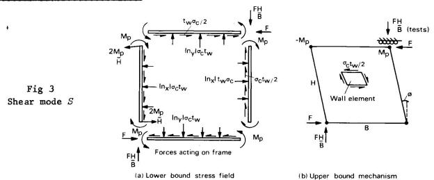
All modes will be examined with equal plastic moments in the beams and columns. The assumed mechanism (Fig 3b) has a dissipation of energy in the frame of  $4Mp\phi$  provided that the joints are rigid. For small displacements a rectangular frame would not require any extension of the panel only pure shear. Reference to the yield criterion, Fig 2, shows that the stress point associated with a strain-rate  $(O, O, -\phi)$  is
