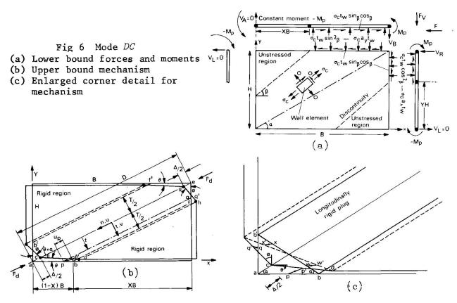
global equilibrium requirements unless a band parallel to the panel diagonal is assumed resulting in a very restricted set of panel parameters for which the solution is valid. Thus a more general solution free from these restrictions, is required and is currently under investigation. Where the solution is valid X, Y and f are given by
