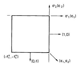
Fig. 1 Yield Locus for Concrete in Plane Stress.
