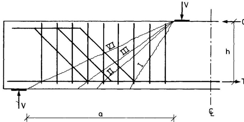
Fig. 4 Reinforced Beam with Stirrups and Bent-up Bars.
