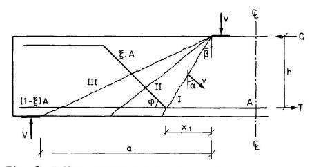
Fig. 2 Failure Mechanisms for Beams with only one Bent-up Bar.
