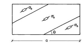
Fig. 2. Stress field in concrete with low degree of reinforcement.
