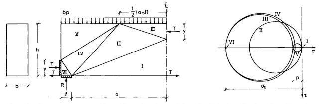
Fig. 5. Beam under consideration showing adopted division of concrete into adopted division of concrete into zones with homogeneous stress fields.
