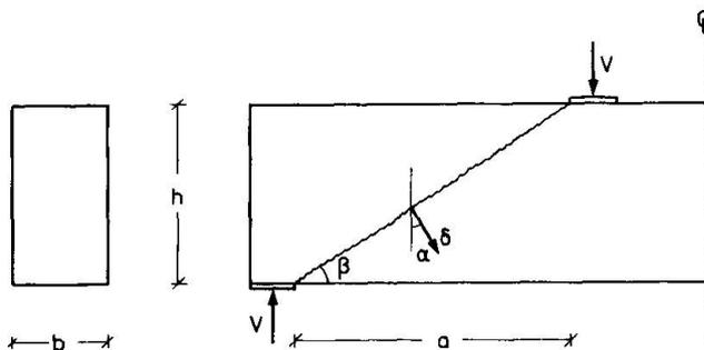
Fig. 11. Alternative failure mechanism for  $\pi = 0$ .
