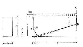
Fig. 7. Failure mechanism used.
