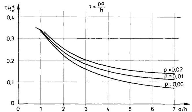
Fig. 16. Variation of carrying capacity with  $\rho$  and  $\frac{a}{h}$ .
