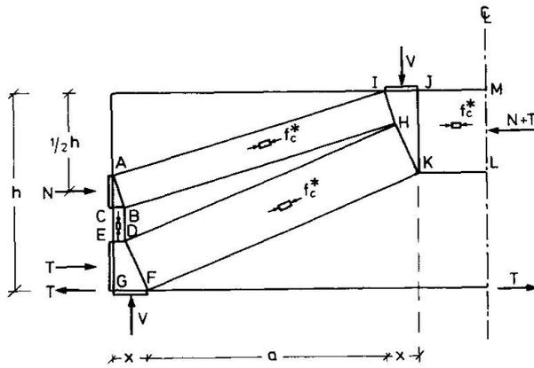
Fig. 9. Stress distribution for use in lower-bound solution.
