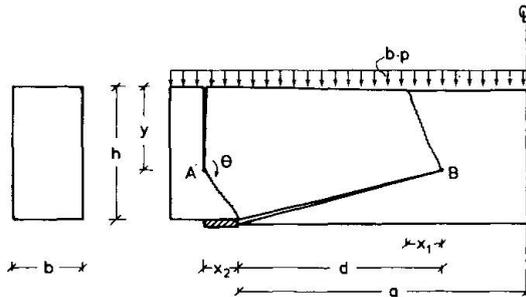
Fig. 15. Failure mechanism.
