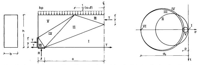
Fig. 5. Beam under consideration showing Fig. 6. Mohr's circles for the stress adopted division of concrete into fields in the zones from fig. 5. zones with homogeneous stress fields.
