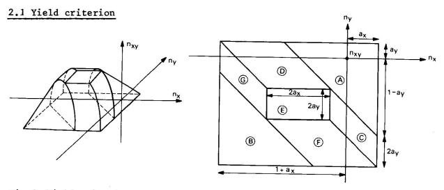
Fig 2 Yield criterion for orthogonally reinforced panel elements
