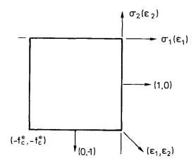
Fig. 1 Yield Locus for Concrete in Plane Stress.
