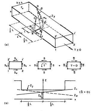
Fig. 5 Effect of Warping Restraints
