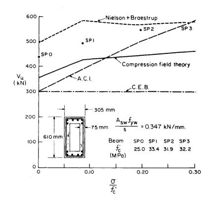
Fig. 7 Shear Capacity versus Level of Prestress
