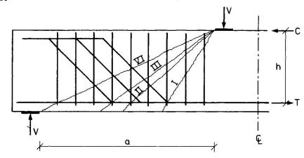
Fig. 4 Reinforced Beam with Stirrups and Bent-up Bars.
