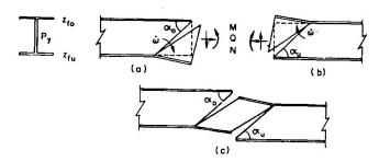
Fig. 3 Collapse Mechanisms for Underreinforced Beams in Bending and Shear
