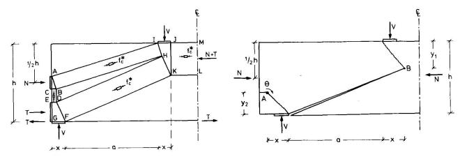
Fig. 9. Stress distribution for use in lower-bound solution.
