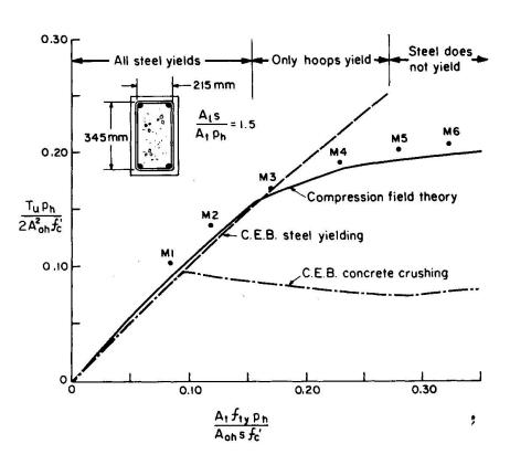
Fig. 6 Torsional Capacity versus Amount of Reinforcement
