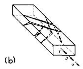
Fig. 4 Basic Torsional Collapse Mechanism (a) and Combined Mechanism (b)
