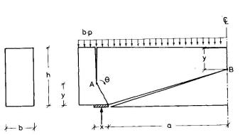
Fig. 7. Failure mechanism used.
