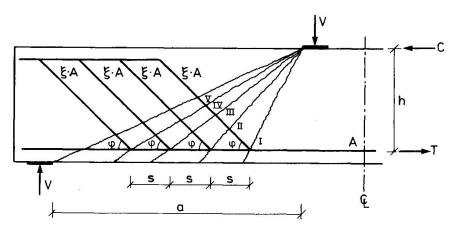
Fig. 3 Failure Mechanisms for a Beam with several Bent-up Bars.
