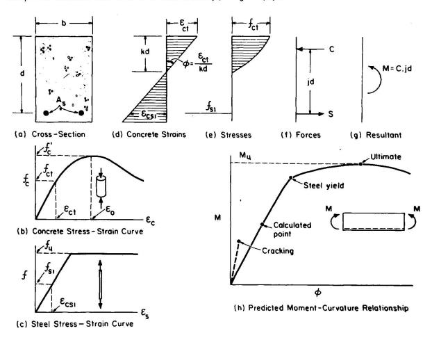
Fig. 1 Plane Sections Theory for Flexure
