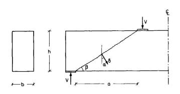
Fig. 11. Alternative failure mechanism for  $\pi = 0$ .
