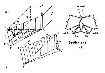
Fig. 6 Basic Torsional Mechanism for Solid Beams
