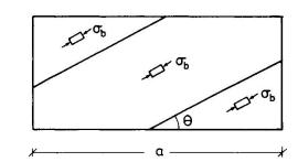
Fig. 2. Stress field in concrete with low degree of reinforcement.
