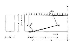
Fig. 15. Failure mechanism.
