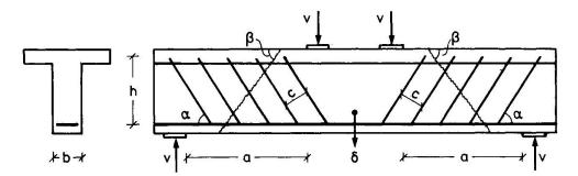
Fig. 1. Beam under consideration, showing failure mechanism.
