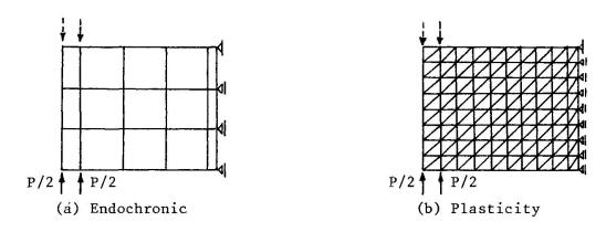
Fig.7 Finite element idealizations of Cervenka's shear panel
