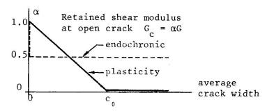
Fig.3 Shear retention factor
