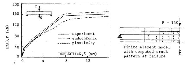
Fig.5 Results from analyses, Burns-Siess beam
