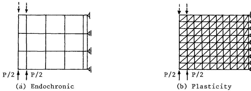
Fig.7 Finite element idealizations of Cervenka's shear panel
