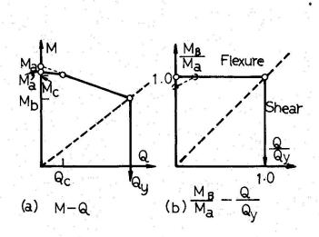
Fig. 5 Moment-Shear Force Interaction
