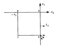
Fig. 2 Yield Criterion for Concrete
