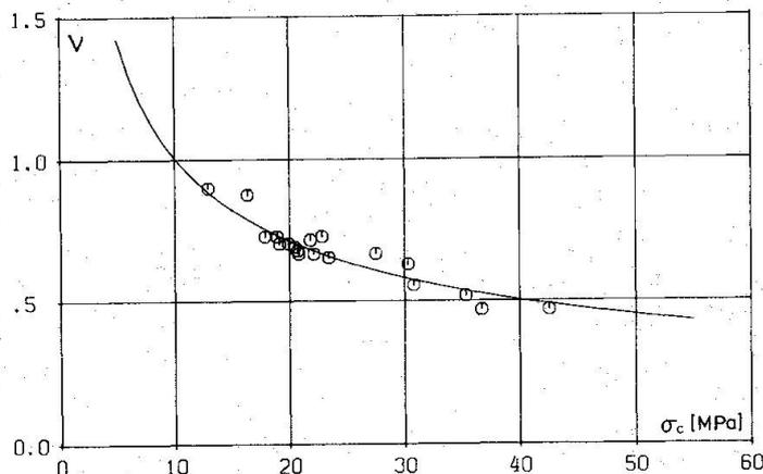
Fig. 4. Empirically determined  $v$ -curve:  $v = 3.2/\sqrt{\sigma_c}$ ,  $\sigma_c$  in MPa and test results from [79.1]
