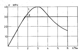
Fig. 2. 1:The analytical stress-strain curve.
