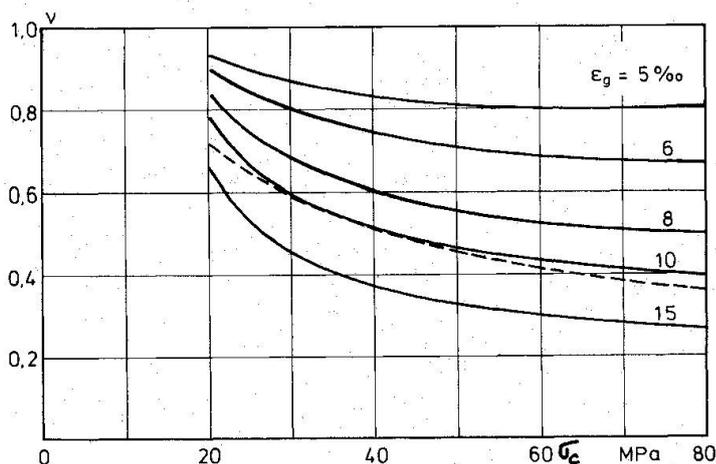
Fig. 3.  $v$  as a function of  $\epsilon_g$  and  $\sigma_c$ . The dashed curve<sup>g</sup> is the curve  $v = 3.2/\sqrt{\sigma_c}$ ,  $\sigma_c$  in MPa from fig.4.
