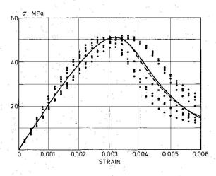
Fig. 1. Measured stress-strain curves
