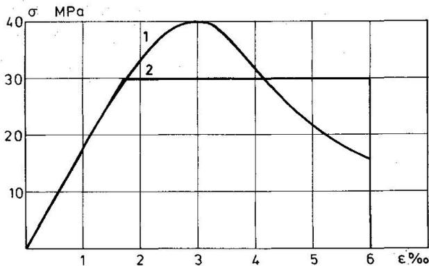
Fig. 2. 1: The analytical stress-strain curve.
