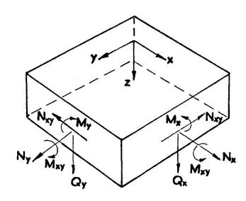
Fig. 1 Sign convention for stressresultants on a slab element
