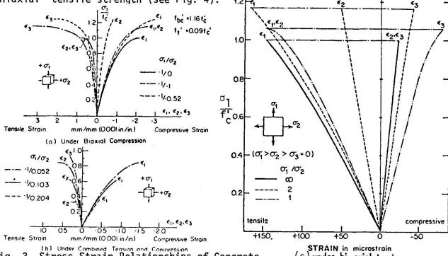
(b) Under Combined Tension and Compression Stress-Strain Relationships of Concrete
