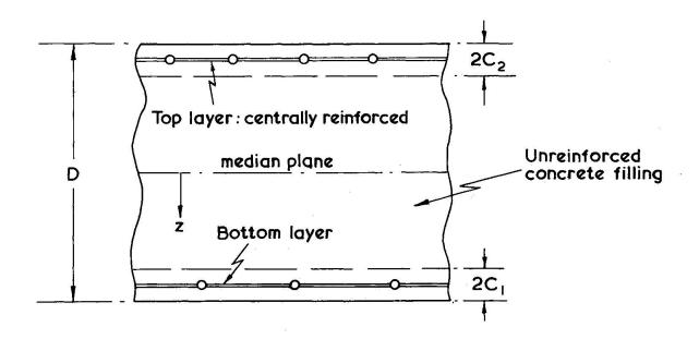
Fig. 8 Filled-sandwich model of a slab element
