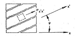
Fig. 9 Pattern of Cracks and Stress Distribution in a Cracked
