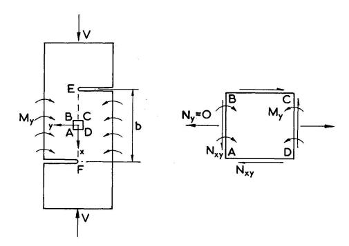
Fig. 9 Assumed stress conditions in 'push-off' test specimens
