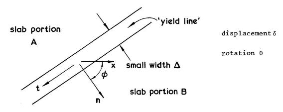
Fig. 5 A yield line between two rigid slab portions
