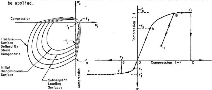
Fig. 11 Loading Surfaces of Concrete in Biaxial Stress Plane.
