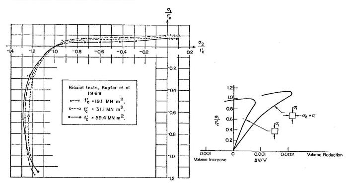
Fig. 4 Biaxial Strength Envelope of Concrete.
