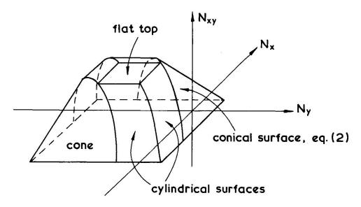
Fig. 6 Yield surface for orthogonal reinforcement, membrane forces only
