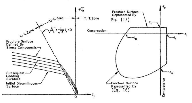
Fig. 6 Loading Surfaces of Concrete in  $(I_1, \sqrt{J_2})$  Space.
